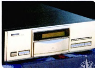
The retail PD-95 looks great, but the prototypes had solid, not pressed aluminium body panels
