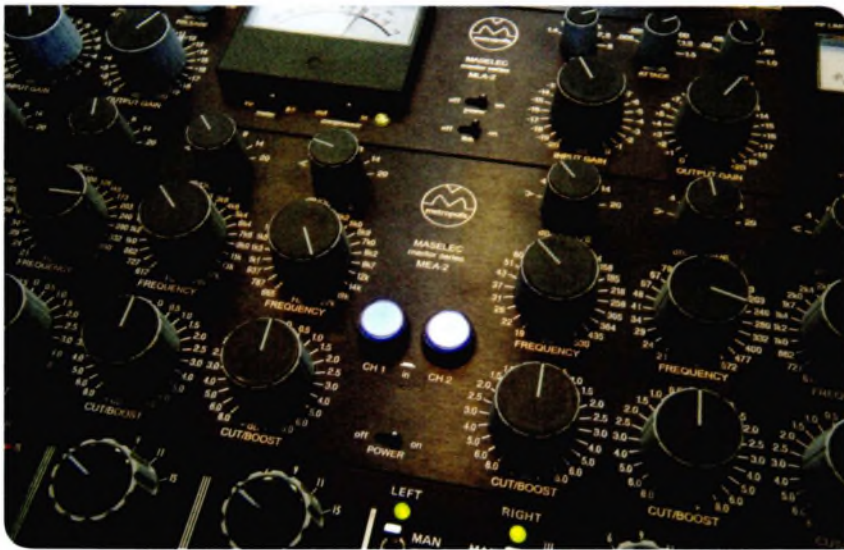
Masalec MAE-2 parametric equaliser on the stereo mixing desk
