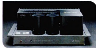
The JVC featured matched pairs of reservoir caps
