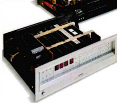
The ST-910's main PCB with its daughter boards
