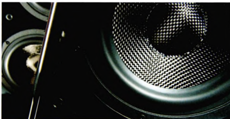
Multiple passive drivers are included by Teufel as an alternative to reflex port loading. The result is a sound with less distortion over a broader volume range
