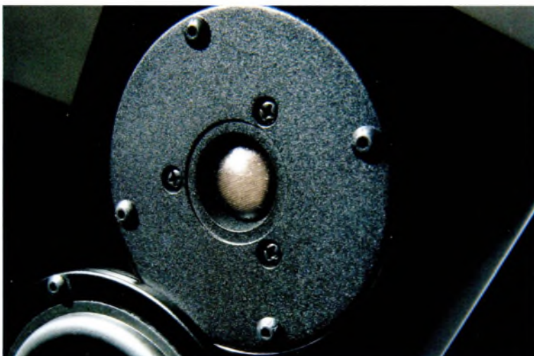
The 19mm doped-fabric dome tweeter and the bass/mid driver are located close together which complements the use of a slim cabinet enclosure
