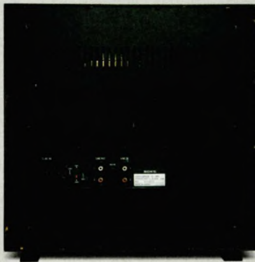
How we used to live – typical late seventies Sony back panel, with RCA phono socketry next to the (then) obligatory 5-pin DIN
