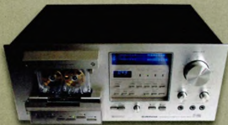
Full metal jacket: 1980 model-year high end decks like this Pioneer CTF-950 boasted Type IV metal tape compatibility, for improved dynamic range...
