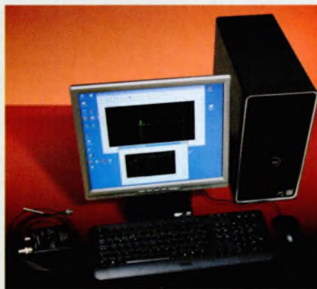
Measurement computer runs ARTA software for frequency response testing and LIMP software for impedance testing, plus custom-written code for post-processing of the results
