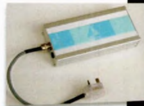
Taga distribution block and Silver Jaya mains filter that plugs into a spare socket
