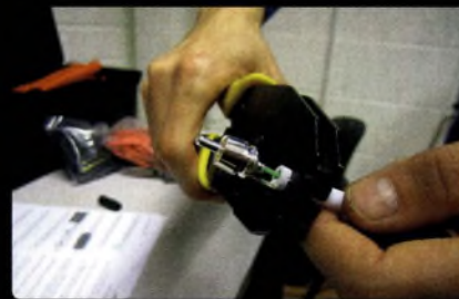
4 The outer part of the plug is squashed around the dielectric for extra robustness
