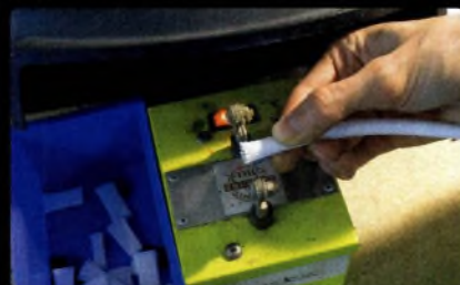
5 The cable's outer sleeve is heat-cut using this special machine, readying for fitting
