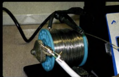
3 The ends of the conductors are threaded to the plug, which is then hand soldered
