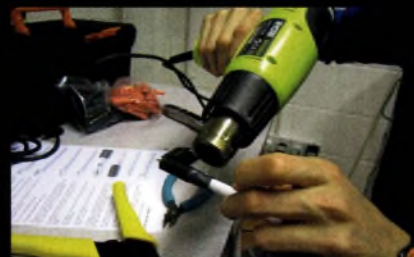
6 The sleeve is pulled up to the end of the plug, and heat shrink is fitted using a special heat gun
