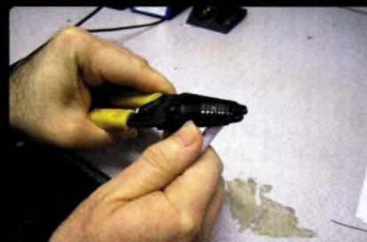
2 The shielding is trimmed away using sharp pliers and then the ends of the conductors stripped away
