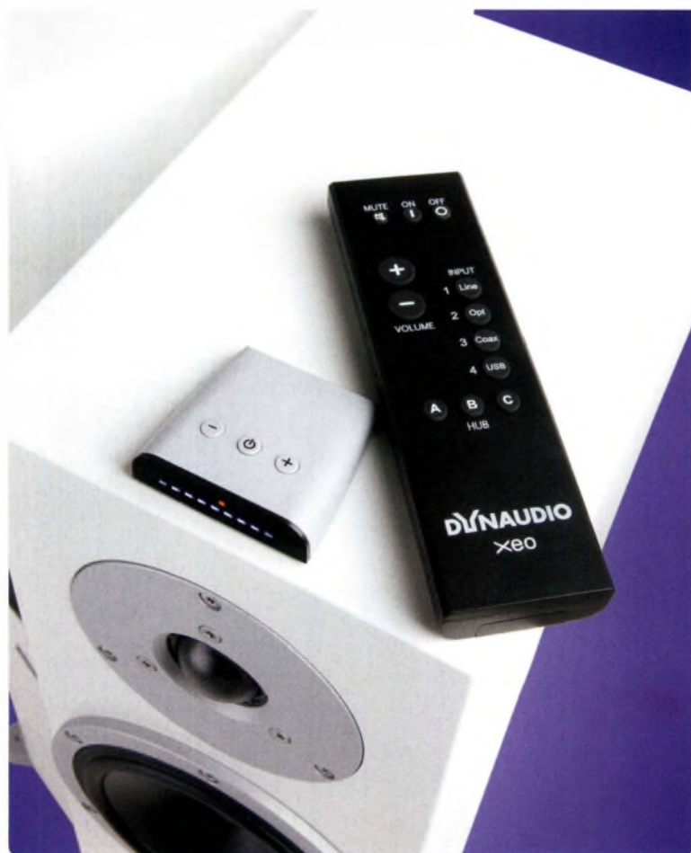
The remote sensor and control panel on top of each speaker shows volume level via a row of LEDs
