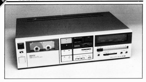
The Denon DR-M2 is clearly a 'budget' threehead deck, as it offers off-tape monitoring but is not cluttered with relatively rarely-used additional facilities. Encased partly in metal, partly in plastic, it is handsomely styled with almost all the tape deck functions behind a plastic membrane on the front panel.
