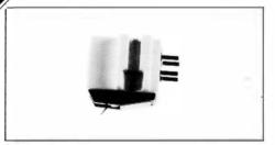
The 303 is a notable member of a new and costly group of moving-coil cartridges. A relatively low mass model at 5.8g, it has unnecessarily high compliance of 44cu, resulting in a recommendation for use with low mass damped arms only.
