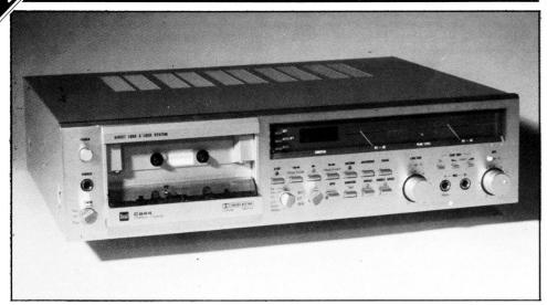
This top-of-the-range deck from Dual has both Dolby *B* and *C* noise reductions systems, offers two tape speeds and incorporates a combination head which allows off-tape monitoring. Phono line inputs and outputs on the rear panel are complemented by a five-pole DIN socket to normal DIN specification, with an additional DIN socket giving an off-tape monitoring signal. Separate friction-locked rotary record level controls are provided for line/DIN and mic inputs, thus allowing mixing if required.
