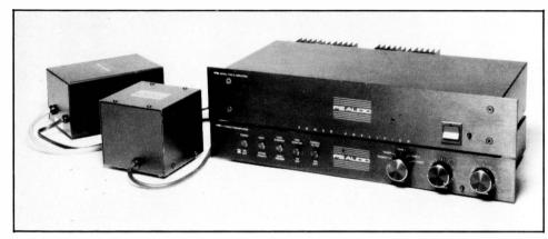
A respected American-made amplifier system. the PS Audio range offers several possible options. We chose the model IV, a comprehensive pre-amplifier which includes a passive control option for high level sources, plus the 50W Two C power amplifier.
