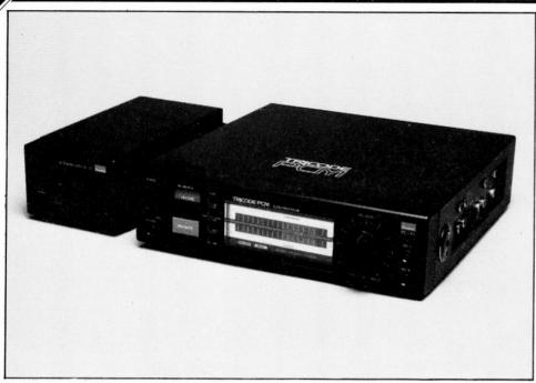
Sansui's first digital adaptor, unusually, or playback and so it is not possible to code switch selecting appropriately. and de-code at the same time. The PCX1 will allow copying with error correction, but not down to analogue and back again. It only has 14-bit resolution, but good dither was provided. Sonvs.
