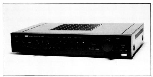
A budget model, the 101 is specified at 30W per channel and comes in a low, slim-profile satin black case. Tidily presented, the front panel offers a headphone socket, speaker muting, bass and treble controls, a high frequency filter, and selection of inputs: these are tape 1 and 2, aux/CD and tuner. A loudness contour switch is also provided and there are coloured lamps to show which input function is selected.
