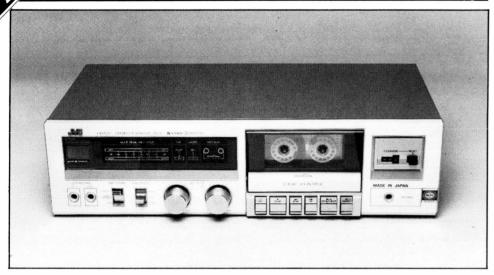
Very modestly priced, the JVC KV-22B does incorporate both B and C Dolby noise reduction systems and is completely encased in metal. In other respects, this two-head deck is very basic. Line in/out phono sockets are clusted together on the rear, and the mains lead is, as usual, a two-core captive one. Two separate rotary record-level controls are provided for left and right inputs, and as these are spaced apart horizontally, they were easy to use, but difficult to bring up precisely together.
