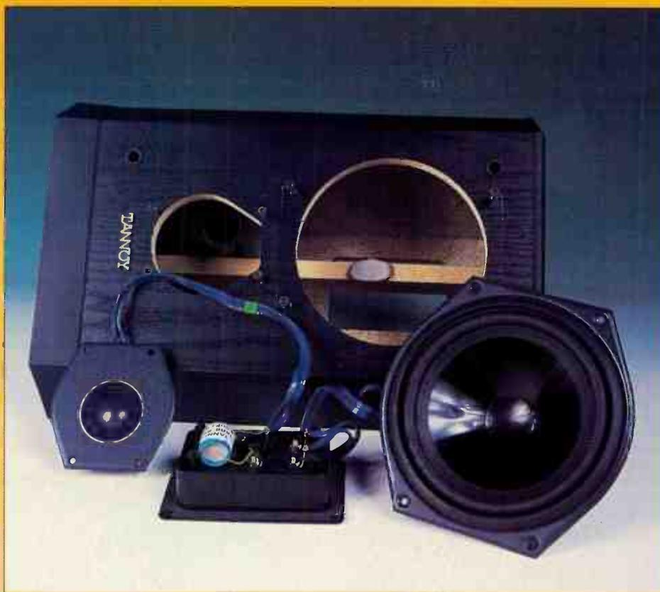
◀ The component parts of Tannoy's 'Limited Edition' 605 loudspeaker. Note the attention to detail, damped Ansar Supersound crossover capacitors, Audioquest internal wiring, central bracing strut which clamps the bass unit via a piece of Bluetak and lead-massed top and bottom plates.
