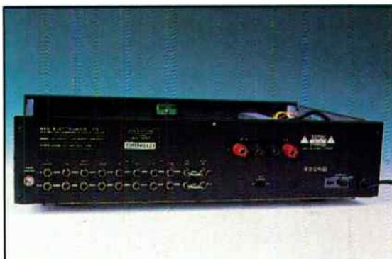
**Behind the 302. Both impedance and 'Soft Clipping' switches are visible. Also to be seen are the links which separate pre and power sections of the amplifier.**
