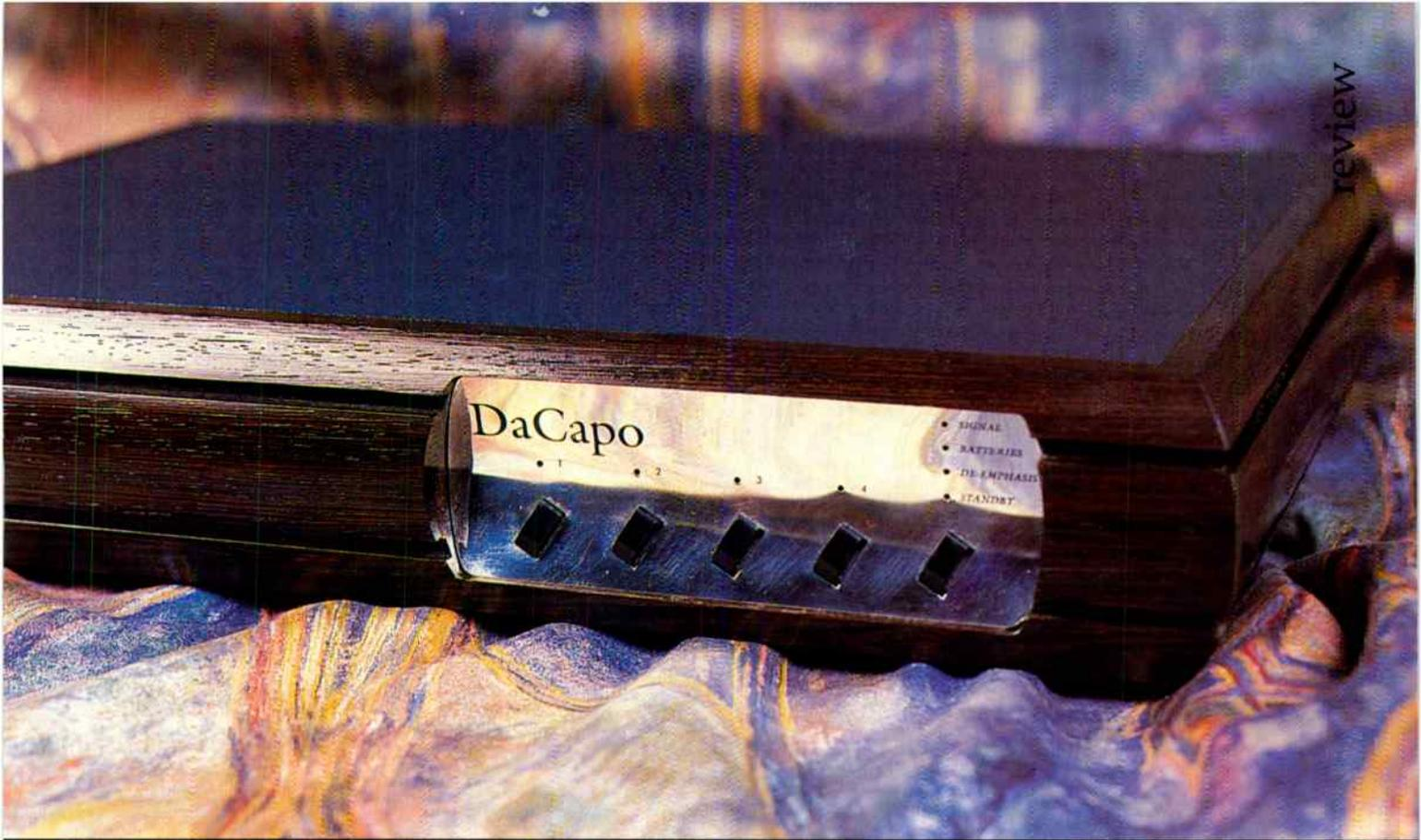
In addition to a BNC co-axial digital input from a CD transport, there are also three further spaces for plug-in digital input and output options, known as Digital Interface Cards. This allows some flexibility. At present, most domestic users only need a convertor for Compact Disc reproduction. In future, however, the Da Capo could accept further digital signals, such as Digital Audio Broadcasts, together with an actively reclocked datastream for output to any digital recording medium.
