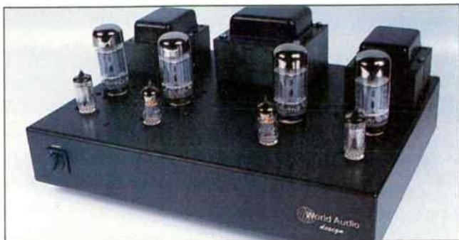
Here's a superb, Class A, 20watt stereo power amplifier that uses the inexpensive Russian 5881 output valve, a military version of the regarded American 6L6, designed for low distortion audio work. It has super-quality output transformers (4/8/16Ω selected internally) to minimise distortion and the input stage uses triode working. A rugged, sixteen-gauge, all-welded steel chassis is provided, together with protective bottom plate for safety; a protective top cover is an optional extra.
