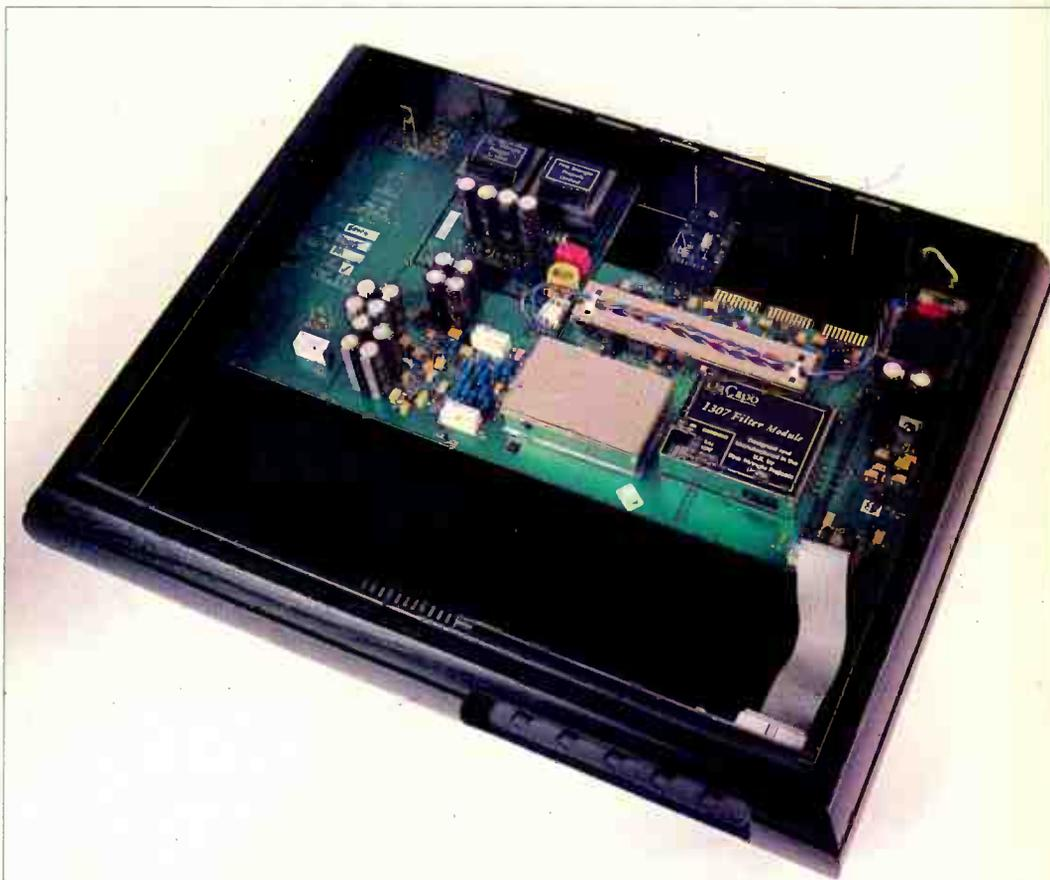
Da Capo uses high quality surface mount components and a modular approach to allow future upgrades with ease.
