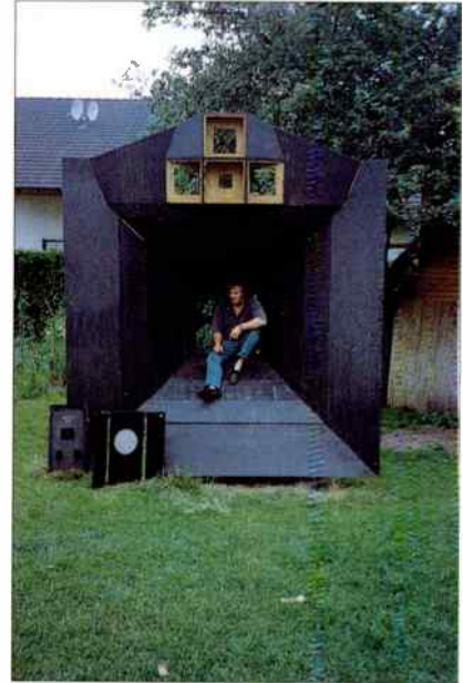
Ahrens Audio have a 12 foot-tall straight tractrix horn.
