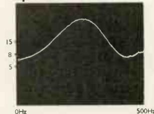
The peak in the impedance plot indicates that the resonant frequency of the driver is 26Hz.
