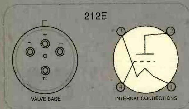
meant for modulation service in transmitters and other very high-power professional applications. You would have to be totally mad to build an amplifier using one for the home. The heat emitted would be tremendous, especially in a small room: the filament alone burns up over 90 watts, so two 212Es in full flight would put out 730W of heat. The bulb would be a positive health hazard, searing the skin at a touch. However, the 212E is very popular in Japan.
