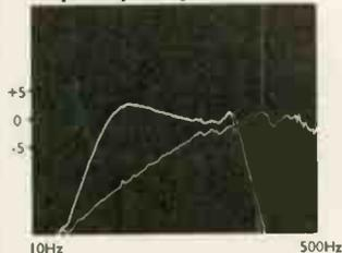
Electronic equalisation lifts the driver's output by 6dB/octave
