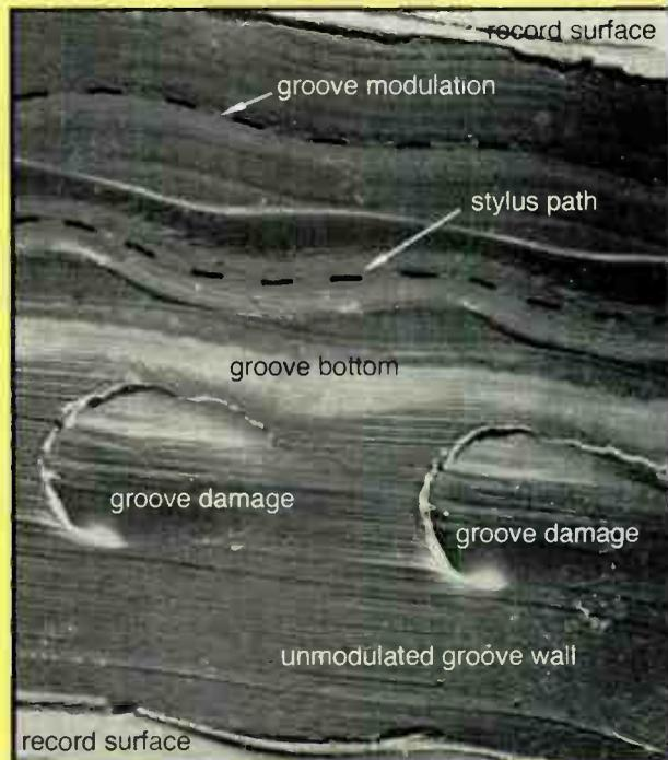
Here is the damage caused to a record groove by mistracking. The stylus has ploughed a signal into the top wall and pitted the bottom wall, causing permanent damage.
