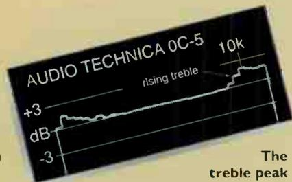
The treble peak which contributes to the AT-OC5's bright sound is clearly visible here. Ortofon's MC 10 has a flatter response.
