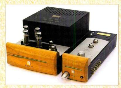
The Power 35 produces 35 watts from a pair of EL34s working in push-pull to give what the importers UKD describe as a lush, liquid and transparent sound.
