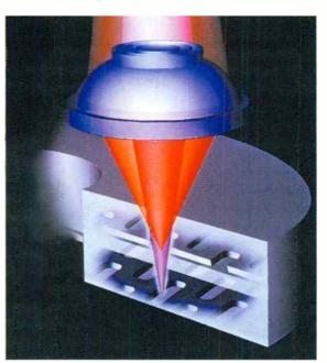
The dual-focus pick-up allows the DVD-A350 to read double-layer DVDs.
