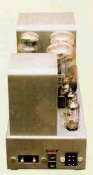
On the Quad II's rear panel are the mains input (left), 'speaker terminals (centre) and Jones connector (right).
