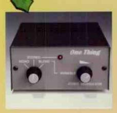
without needing an additional amplifying stage and the effect it can have on the sound. If there is insufficient signal for decent stereo, the beacon fails to light and you have the options of switching to mono for lower noise or maybe using the handy Blend control to pick an optimum in-between point. Tuning in to Radio 3 for what is probably the least meddled-with
