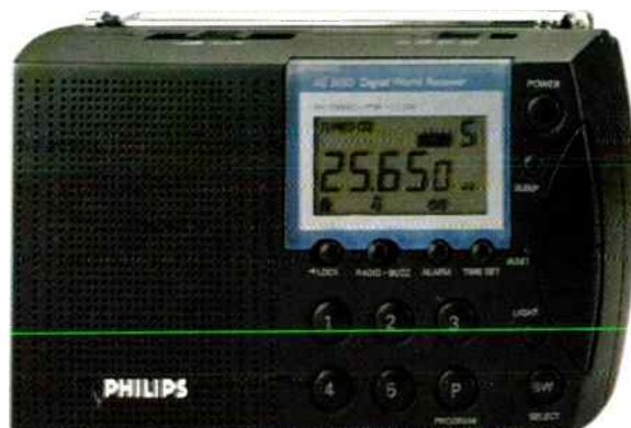
A 'Digital World Receiver' from Philips. This is an analogue radio with digital tuning.
