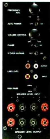
The Entry S subwoofer has a comprehensive control panel with good features
