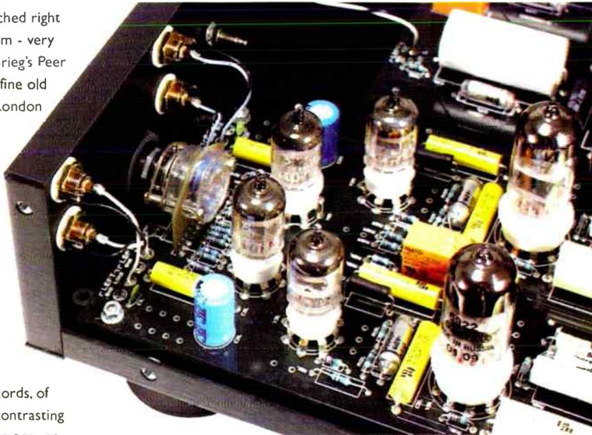
**The GM 70 uses PC900 valves in the input stage and 6922 valves for the gain and output stage**
