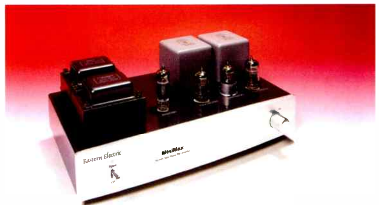
Eastern Electric Minimax valve phono stage - a great sound from moving magnet and moving coil cartridges. Note the big audio transformers for moving coil cartridges.
