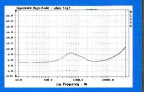
Impedance of the H1189 treble unit shows the broad, well damped fundamental resonance of the unit due to ferrofluid damping and the rear enclosure used on this unit.
