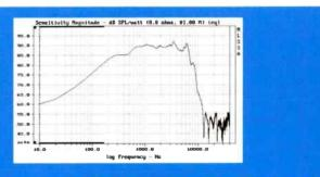
With H1217 in an enclosure with a 20cm wide baffle the baffle step becomes clearly visible. Ignore the response below 200Hz as the gating is not wide enough to show any accuracy down here, as shown by the black bars.
