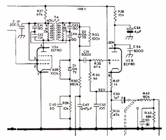
The composite stereo signal, comprising mono + stereo subcarrier can be picked up at T4, One Thing told us. I used the high level point shown by our red arrow. Note this is at 85V and may give a small belt (I didn't try it!), so exercise caution if you do this yourself. Best to let One Thing instal and set up.
