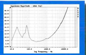
The impedance plot of H1217 shows the typical double hump of a bass reflex tuned to 40Hz. Ignore the triangular look of the peaks which is because the number of points plotted down here doesn't provide high accuracy. The wrinkle in the trace at 300Hz indicates an enclosure resonance (well damped). Another wrinkle at 800 Hz is part of the drive unit characteristic. We know this because it can be seen when the impedance is measured outside the enclosure.
