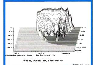
'Waterfall' delayed resonance graph of H1217 in its enclosure. The ridges at 3500Hz and 6000Hz correspond to peaks in the frequency response graph and indicate minor resonances in the drive unit.
