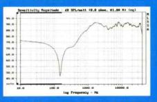
H1189 in the enclosure doesn't look much like the manufacturer's spec, does it? The dip between 3 – 6kHz is partly due to the proximity of the cabinet edges and also due to the bass unit cone below It. Again ignore the trace below 200Hz.
