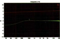
Turning bass down to -1 on the NAD315BEE introduces shelf bass cut. This neatly compensates for wall mounting a large-ish loudspeaker, a scheme with many benefits. Stand mounting is always the best choice though.
