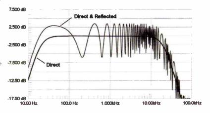
Plots of driver mounted low on baffle, in proximity to floor, showing cancellation and reinforcement effects between direct and reflected sound.
