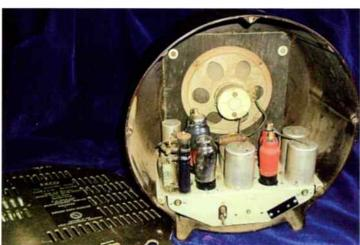
Table radios of the 1930 – 1950 era, such as this EKCO 75, used the deep, bakelite cabinet housing to act as an extended baffle, normally fitted with a perforated back panel for ventilation.
