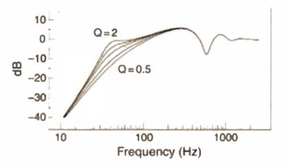
Effect of driver Qts on LF response. As Qts is increased, so is bass output towards the driver free air resonance. A Qts of around 1 is acceptable for an open baffle bass unit.
