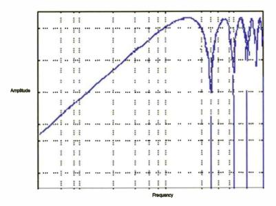
Theoretical plot of driver response on a circular baffle. Note that peaks occur at Fp and its multiples.
