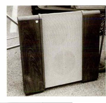
near a side wall – then our 215cm round baffle can generate substantial output down to 40Hz (where it would normally be -6dB measured under anechoic conditions).
