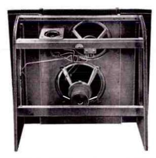
Wharfedale SFB3 rear view. Note cutouts in side 'wings' to reduce resonance and bracing to improve stability. As expected the bass unit is positioned closer to the floor boundary and the midrange unit higher up. A cone treble unit, on its own baffle, points upwards at the rearl
