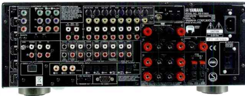
Vertically stacked loudspeaker terminals, not colour coded, but able to accept 4mm plugs as well as bare wires. HDMI inputs and outputs are vertically aligned at far left.
