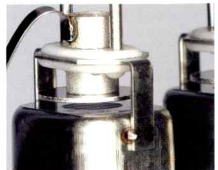
The getter and mica upper support assembly.
