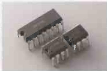
**2SK278B, 2SK78 and 2SJ78 low power static induction transistors used in the B-1a.**
