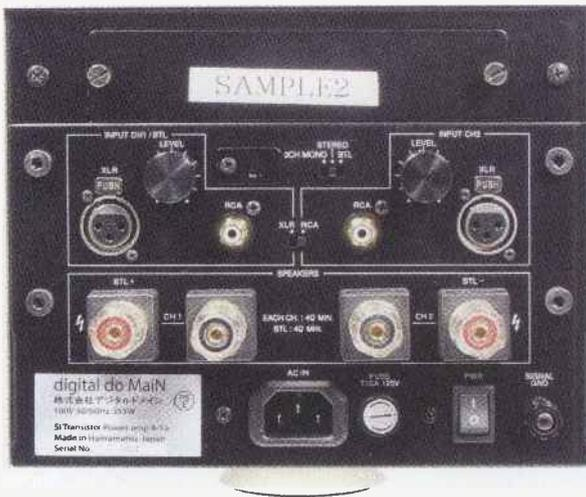
A single B-1a can be set to bridge mode (single channel) to double power. Channel level controls are provided, as well as balanced and unbalanced inputs.
