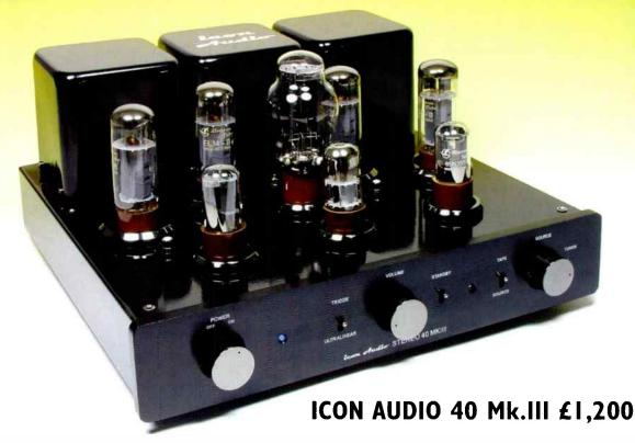
con Audio's 40 has been steadily developed for nigh on ten years, up to Mk III status reviewed here. Although relatively compact at 390x410x210mm, at 25kg it's a big lift. Arrayed on the top of the fascia are the four EL34 (KT88 an option) valves plus one 6SL7/6N9 first stage valve and two 6SN7 phase splitters. Standing proudly in the middle is a Western Electric 274B valve rectifier.
