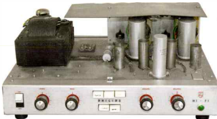
Cover removed, all low level signal valves fully shrouded.
