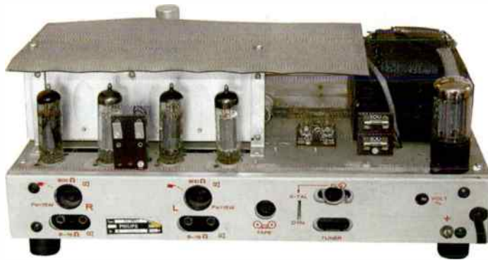
Rear connections; note speaker impedance selector between output valves.
