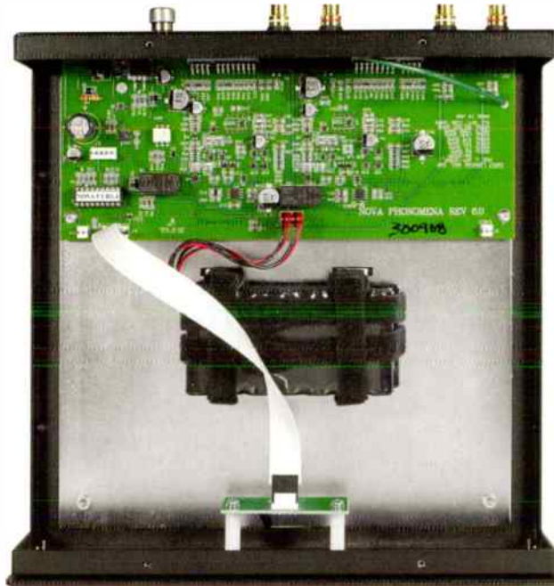
Miniature surface-mount components are used, together with discrete transistors for the audio circuits. A rechargeable NIMH battery provides silent power.
