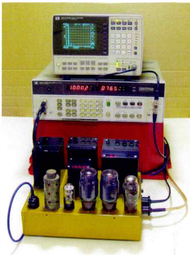
Leak TL12 amplifier under test, the Hewlett Packard 8903A analyser showing 0.0765% distortion, whilst the Hewlett Packard HP3561A spectrum analyser (top) shows it is primarily second harmonic in nature. Not bad for such a venerable old amplifier, proof of Leak's claims, the reason they sound gorgeous – and why they now fetch big prices!
