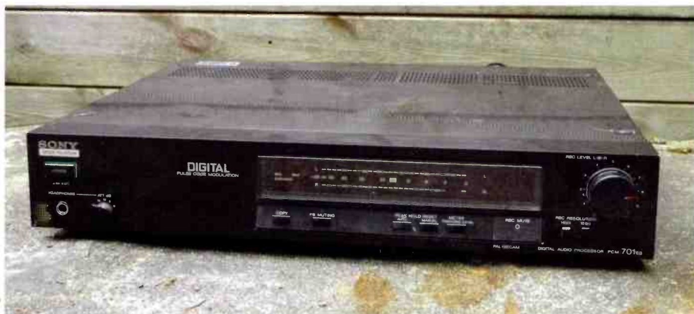
PCM adaptors like this Sony 701ES allowed well-heeled consumers and small studios to make digital recordings for the first time - using commonly-available videotape as the storage medium.
