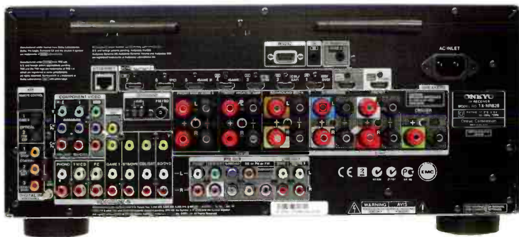
Wi-fi aerials at top supplement an RJ45 ethernet input socket. There are seven HDMI inputs and two outputs. Digital audio S/PDIF inputs, optical and electrical, are at left.
