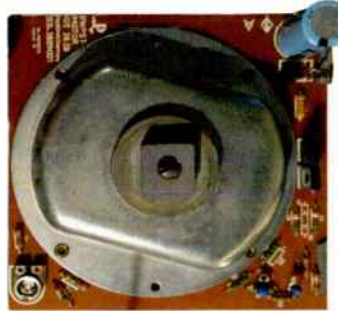
Bottom and top views of the Papst two-phase low-speed-brushless D.C. motor Alan Barnes is using to power a belt drive turntable. But it isn't quartz-locked or phase-locked, says Dave Cawley.
