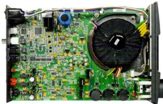
A big linear power supply with circular black toroidal transformer, sits inside DAC-V1. It feeds a web of digital circuitry.
