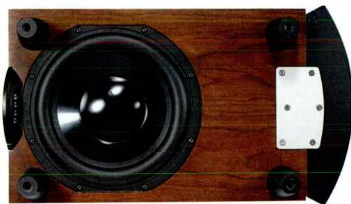
Firing downward is a 10in aluminium cone bass unit, as well as white LEDs for floor illumination. This unit progressively moves out-of-phase with the forward bass unit at higher frequencies to improve matching to the dipole XStat panel.
