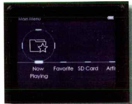
The circle rolls horizontally when the player's jog wheel is turned, to select a drop-down menu.
