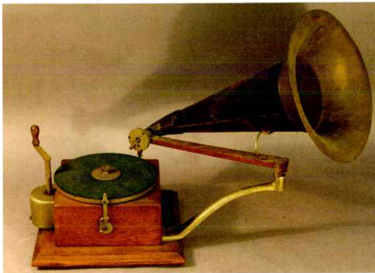
An early Berliner gramophone, driven by a clockwork motor from a sewing machine.
