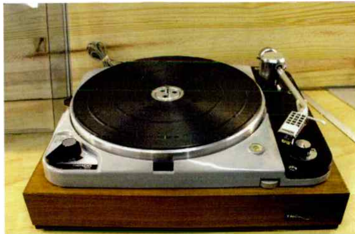
Thorens TD-124 turntable, an idler drive owned by Mario Kopke Tulio.
