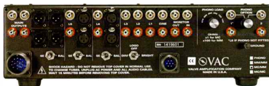
Rear view of the control preamp, MM/MC Phono options and cartridge loading.
