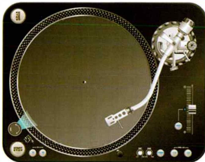
The Hanpin DJ5500 turntable, their top model, uses a 16 pole Direct Drive motor. All lesser models use an 8 pole design that rotates less smoothly. Since most modern Direct Drive turntables are produced by Hanpin, an OEM, their performance will depend upon which motor type is selected. So not all Direct Drives are the same - and not all are good simply because they are Direct Drive.
