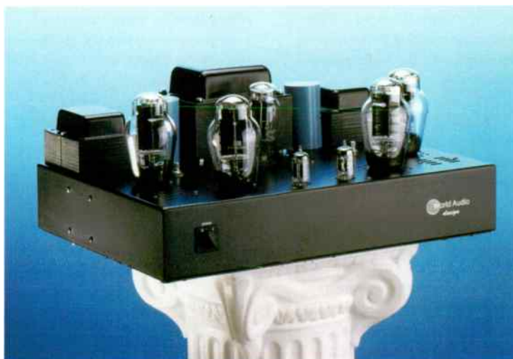
World Audio Design 300B amplifier, designed by us way back in 1993, had switchable feedback. Switching feedback off made it measurably worse - but it sounded better. Oh dear! See what Allen Edelstein says about this.
