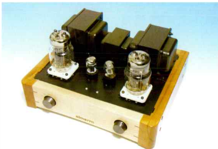
The pretty Almarro SE single-ended amplifier. It uses 6C33C "Russian Trawler" valves that give a bright red glow.
