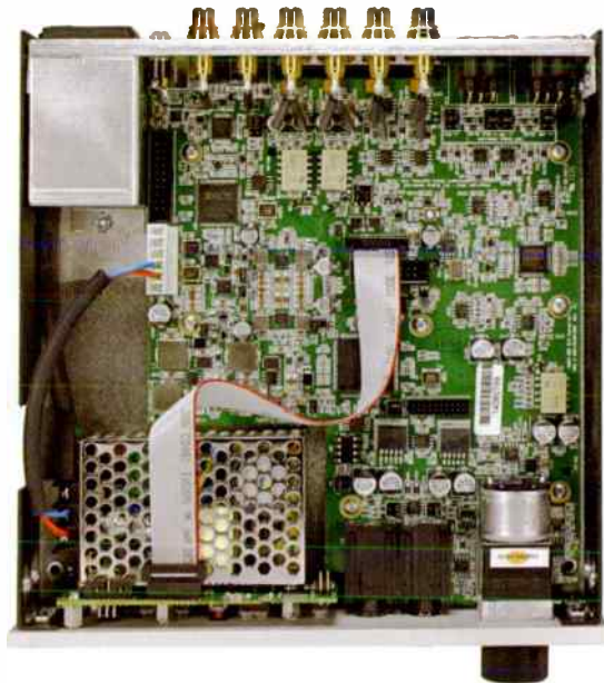
Inside the Benchmark is a screened switched-mode power supply, large output devices that drive any headphones you care to connect, and a motorised volume control.
