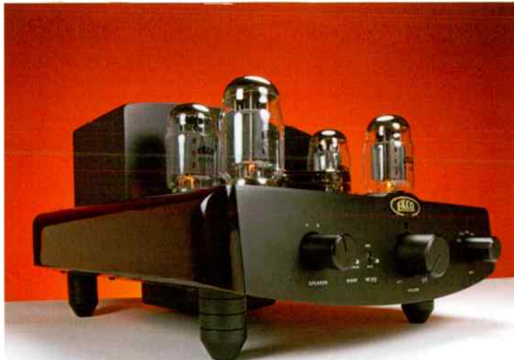
The Ekco EV55 SE amplifier has switchable feedback, labelled 'NF Adj'. "It bothered me that worse measurements sounded better" says Allen Edelstein.
