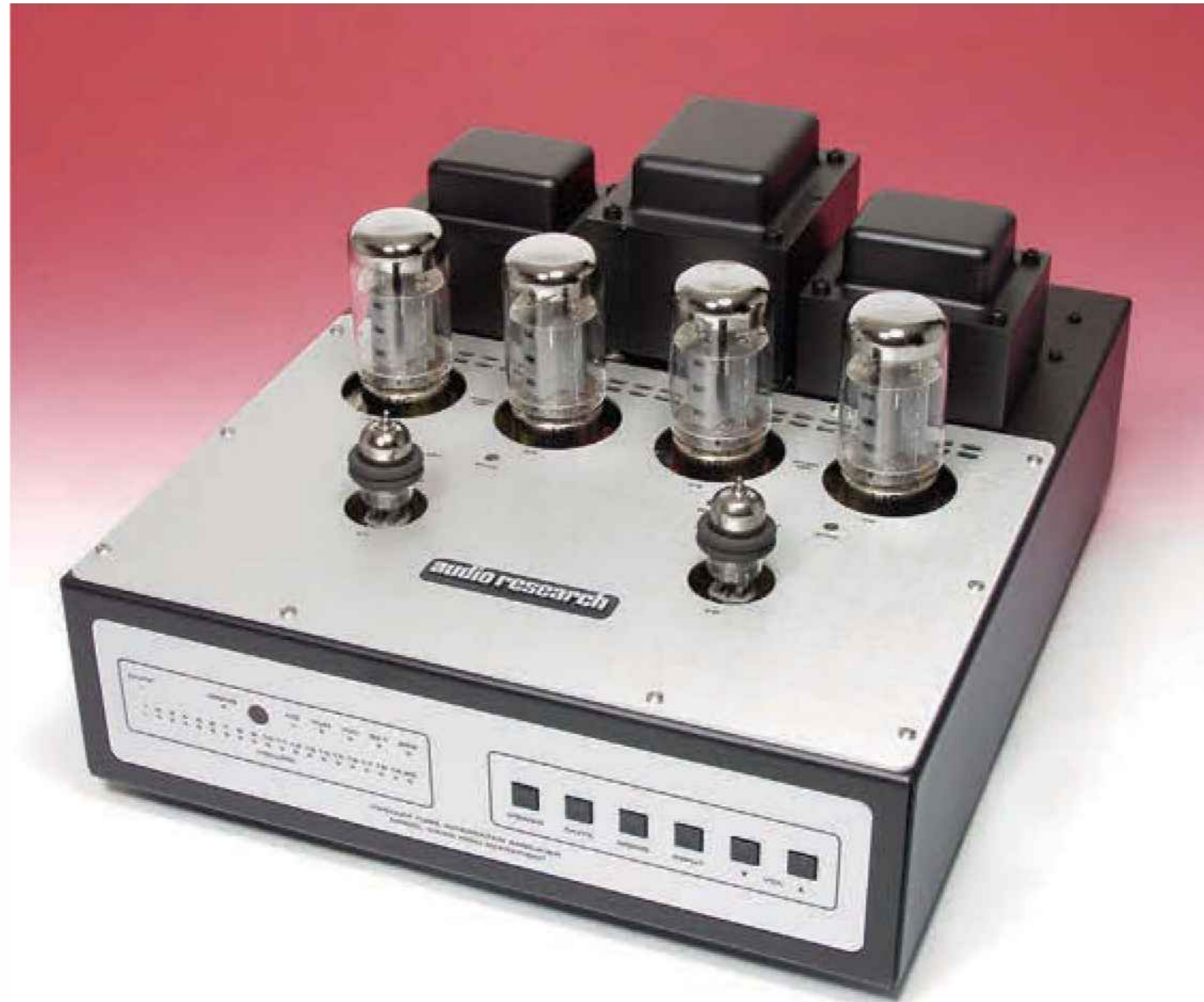
An amplifier that sounds powerful even though it is not: the Audio Research VS60. It's a hybrid in fact, with solid-state pre-amp feeding 6550 output tubes. Well worth hearing.
