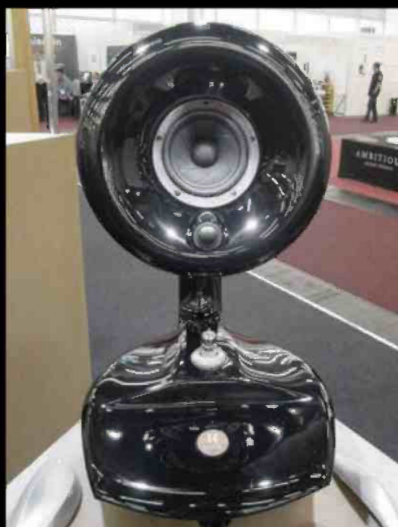
Bluetooth with a difference. Once Audio Design's wireless horn-loaded Su loudspeaker features hybrid valve/solid state for 60 Watts of power, as well as line input and Bluetooth. Oh, and it looks absolutely gorgeous!
