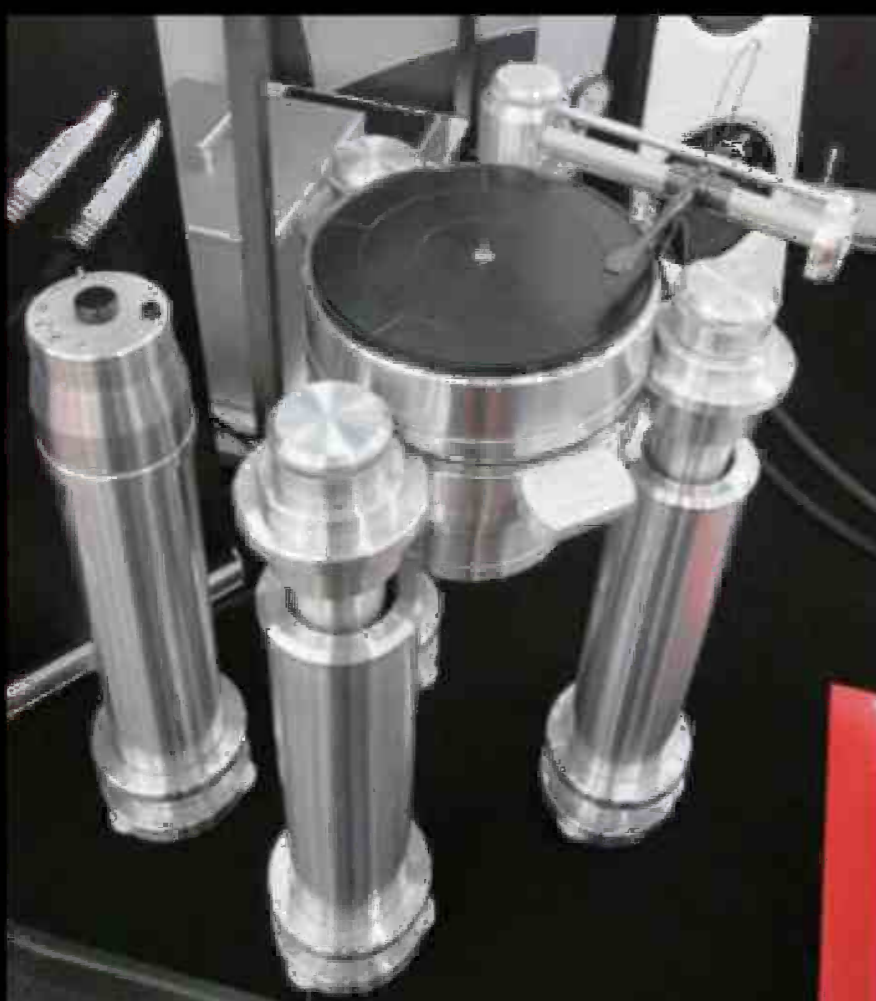
Vyger's massive turntable features high-pressure air bearings for the platter. Really!
