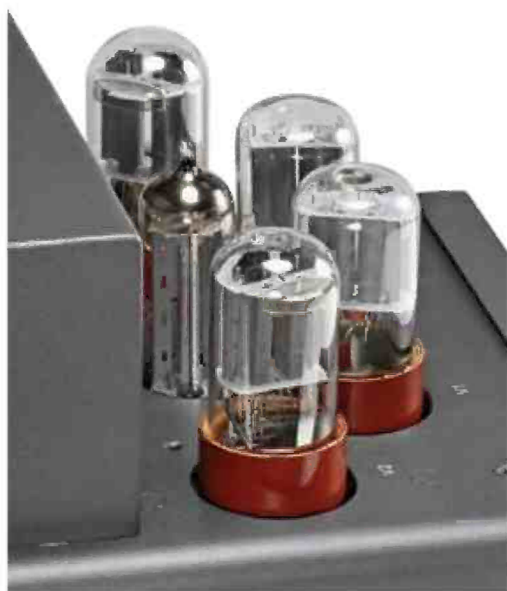
Quad uses pairs of 6SL7 and 6SN7 valves alongside an EZ81 rectifier.
