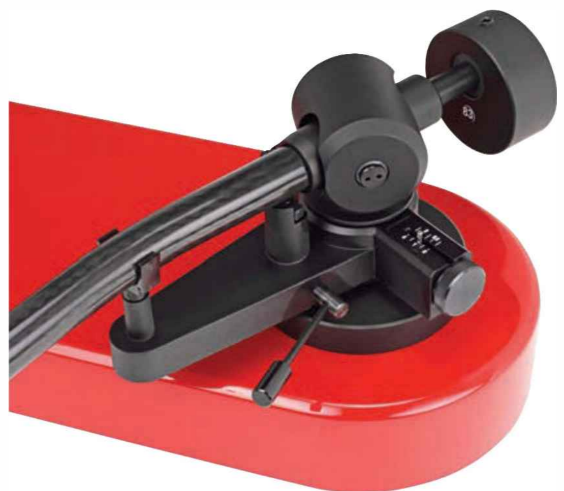
The arm's rear counter-weight uses Pro-Ject's own TPE damping which holds the mechanism in place by using the friction of the rubber mounting bush.
