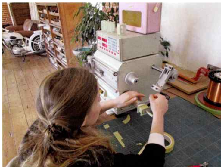
Lucy Gastall at work winding one of the Bespoke Audio Company's custom-built transformers.
