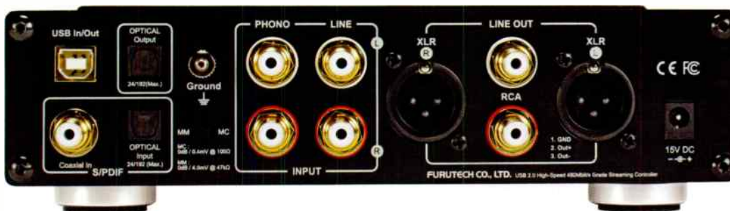
At right sit unbalanced phono socket and balanced XLR chassis plug outputs. There are analogue Phono and Line inputs at centre, plus a small MM/MC slide switch and earth terminal. At left lie digital inputs and outputs.
