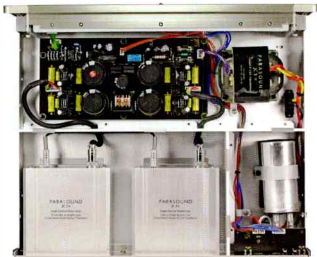
Internal aluminium and steel screens are used to minimise crosstalk, hum and noise.
