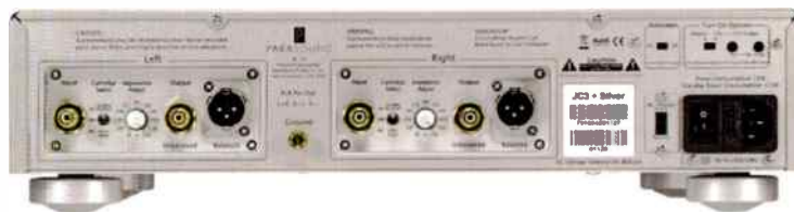
The rear panel carries unbalanced (phono socket) inputs, and both unbalanced and balanced (XLR) outputs.
