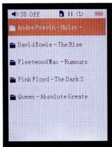
A simple file list on the small screen. Battery charge is at top right, and volume setting at left. Single track repeat is selected here.
