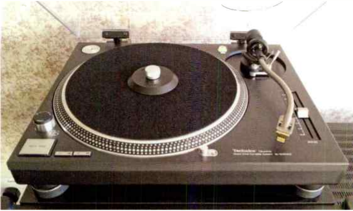
Technics SL-1210 turntable fitted with Alphason Xenon arm by John Taylor-Hartwell.
