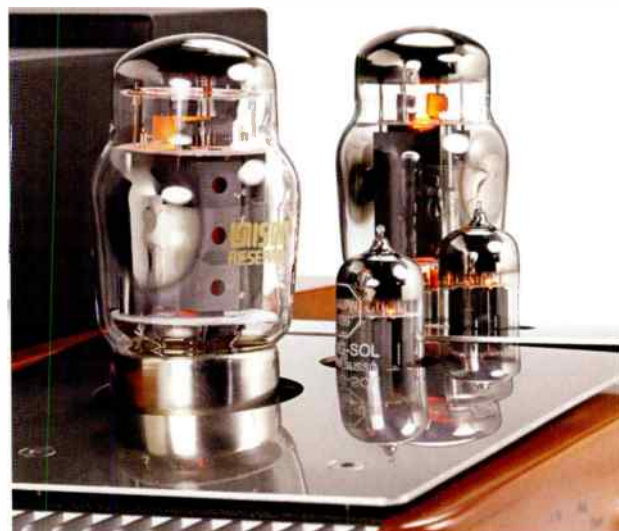
Tubes used on each channel are an ECC82 double-triode (preamp/driver) and a 6550 beam power-tetrode (output). Both of the Tung-Sol branded tubes supplied are made in Russia by the New York-based New Sensor Corporation.
