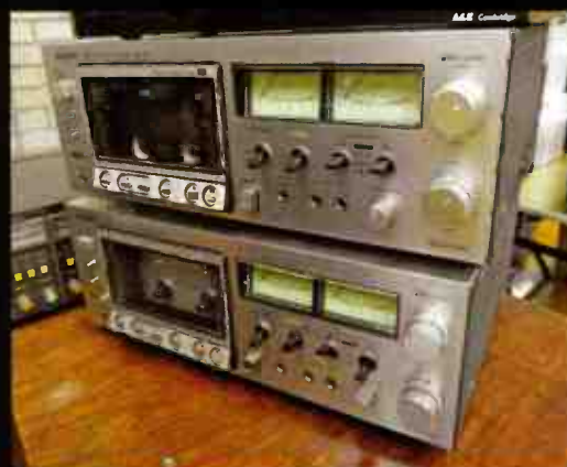
The Elcaset format was designed to combine reel-to-reel sound quality with cassette convenience. Featured a while back in Olde Worlde, it performed superbly but was expensive and arrived too late to make an impact. Few decks were sold and it's uncommon enough to find one machine - never mind the two you see here! This is the 1976-vintage Sony EL-5, a 'budget' two-head brother of the (slightly!) better-known EL-7. £150 was being asked for each one.
