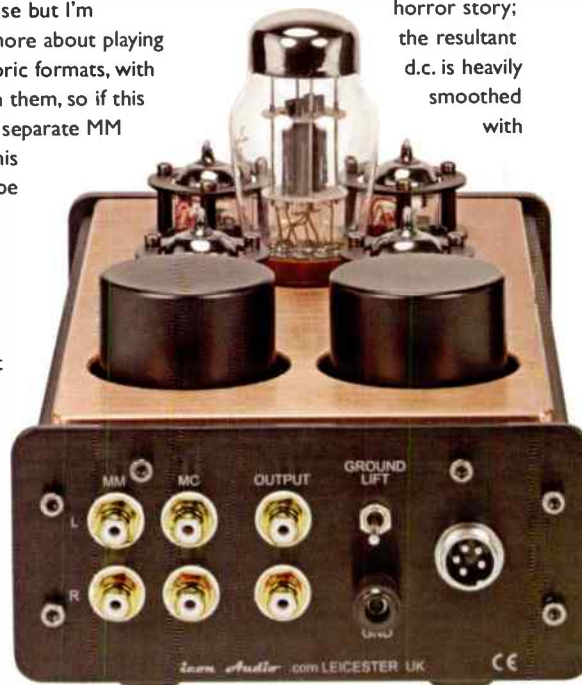
Our rear shot shows gold plated, phono socket inputs and outputs, a ground lift switch to avoid hum, and a ground terminal. The circular canisters are screening cans around the input transformers.
