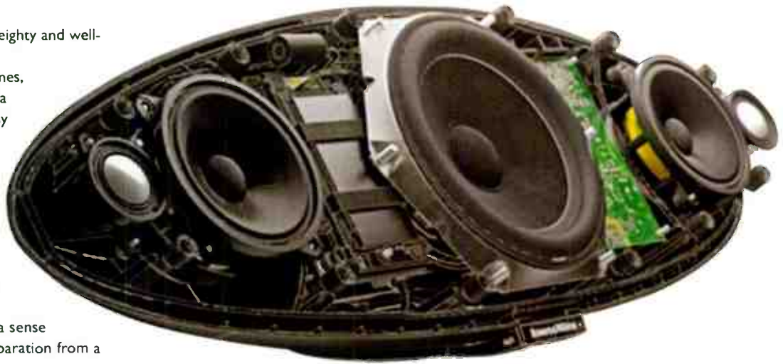
The Zeppelin Wireless driver array consists of two 25mm metal-coated tweeters, a pair of 90mm midrange drivers and a single front-firing bass unit.
