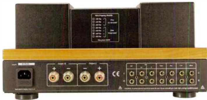
On the right are the (unbalanced) audio inputs, which take the form of gold-plated phono sockets. Note that the windings of the output transformers are optimised for 6-ohm speakers – connected here via high-grade binding-posts that will also take standard 4mm ‘banana plugs’.
