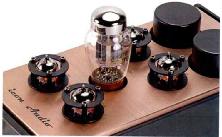
Two low noise ECC88 (6922) twin-triodes per channel provide gain, and a big 6SN7 acts as a low impedance line driver. Input transformers at right step up the MC input. MM goes in direct.
