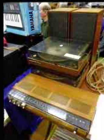
A complete Bang and Olufsen system from the late 1960s - Beomaster 1000 2x15W FM-only stereo receiver, Beogram 1000 belt-idler hybrid turntable (with proprietary cartridge) and Beovox 1000 2-way speakers - was being offered for £20. Many have written off B&O as style over substance, but the Danish firm conducted a lot of original research and development in its Struer lab. Many of its products work exceptionally well. That they look good too is merely an added bonus!
