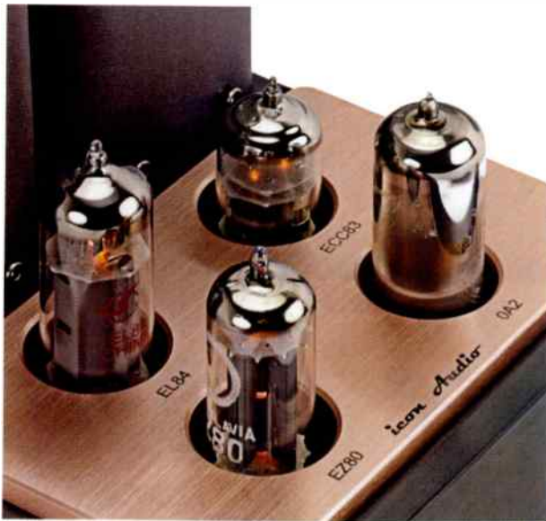
The power supply uses an EZ80 valve rectifier, OA2 voltage stabiliser and both EL84 and ECC83 as voltage regulators.
