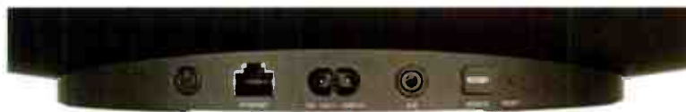
Rear panel connections consist of an ethernet socket, power input, 3.5mm analogue input and USB - although the latter is merely for service purposes.
