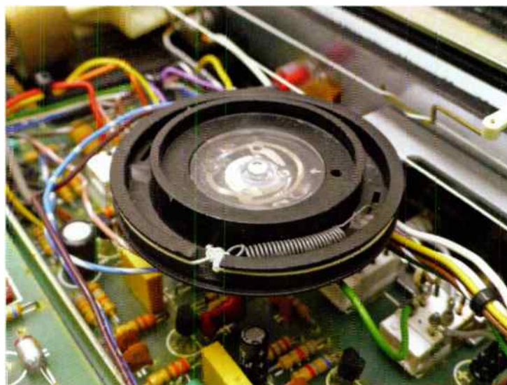
Coupled by drive-cord to the manual tuning system, this is not a variable capacitor. It's actually a precision 100k variable resistor. It's wired as a potential divider, fed from a stabilised 45-volt DC supply. Its output is selected from the switchbank, as an alternative to that from one of the presets, and connected to the varicap diodes that tune this set.
