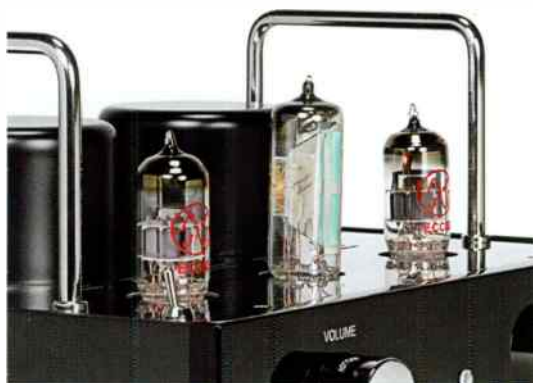
Two 12AU7/ECC82 input valves plus a 6e2 magic-eye indicator valve provide a lovely glowing show - and sound rather good as well. Grab handles also make the Blue Aura easy to manoeuvre - although it is not particularly heavy.
