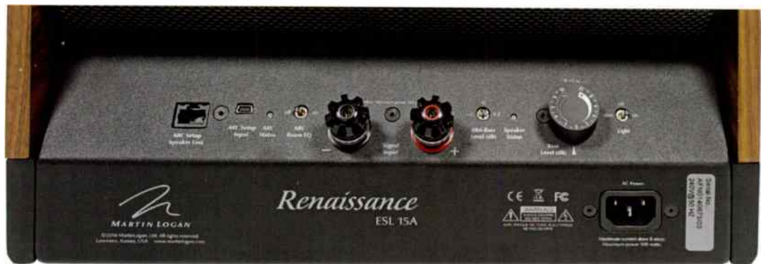
At left are an RJ45 socket for connection during room tuning, a miniUSB input for computer connection and an ARC switch. At right of the input sockets lie a small toggle switch for crossover level adjustment and at far right a light switch.
