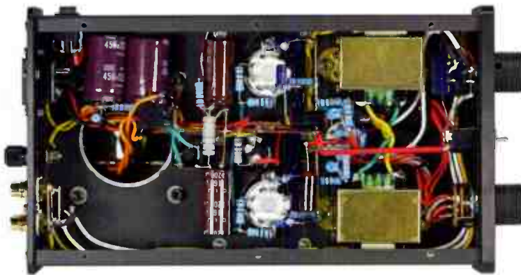
Internally, you can see the unit's output transformers at right. It is hard wired too – there is no circuit board.
