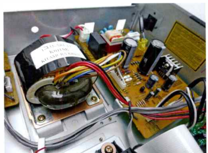
Most mainstream consumer audio products employ switch-mode power supplies. Not so the MDS-JB940 or, for that matter, Sony's entry-level MDS-JE480. Both use a transformer-based 'linear' supply which, although more expensive to implement, tends to be quieter, more reliable and better-sounding.
