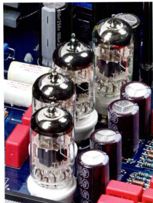
Tung-Sol 12AX7 double-triodes – two per channel – are used in the Unico CD Due's output stage.
