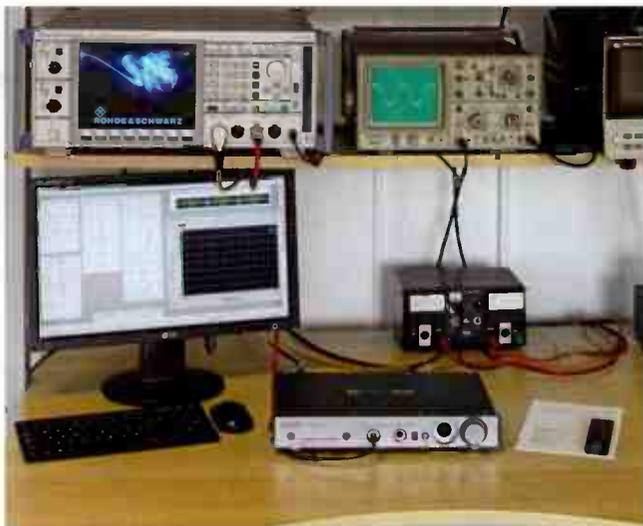
*The Questyle CMA600i headphone amplifier under test, connected to our Rohde&Schwarz UPV audio analyser at top left, with a repeat screen beneath it.*
