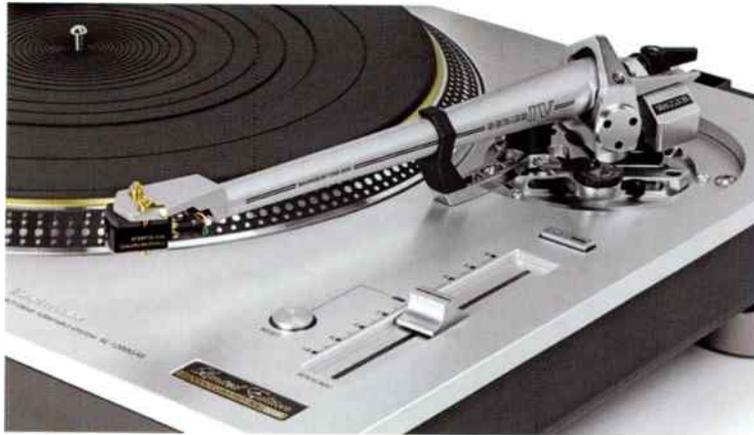
*At the right side lies a turntable speed adjustment slide-control. At centre it provides correct speed, held steady by phase lock against a quartz crystal reference. Total adjustment range is +/-8%, or double that by pressing the oblong x2 button. The SME IV arm is a gorgeous visual match for the Technics.*
