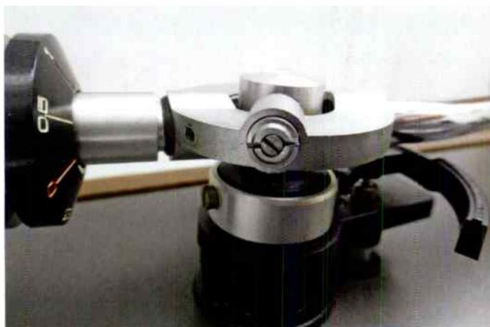
*Hi-fi magazine advice columns of the 1970s were full of 'mods', in the endless pursuit of improved sound quality at any price (and 'free' is always good!). One involved removing the PL-12D tonearm's lateral balance-weight – the mounting post of which screwed into the empty threaded hole visible here; in other words, the owner of our specimen had himself succumbed to 'tweak-fever'! Ironically enough, this weight cannot be seen in the exploded view...*
