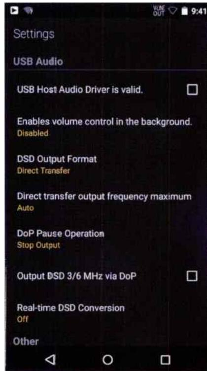
**A formidable array of USB output options, including DSD Direct Transfer to avoid PCM conversion.**
