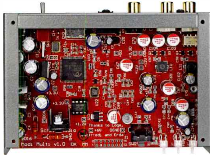
Internally the Modi uses a single Schiit-designed PCB board with the circuit built around an Analog Devices AD5547 multibit chip.
