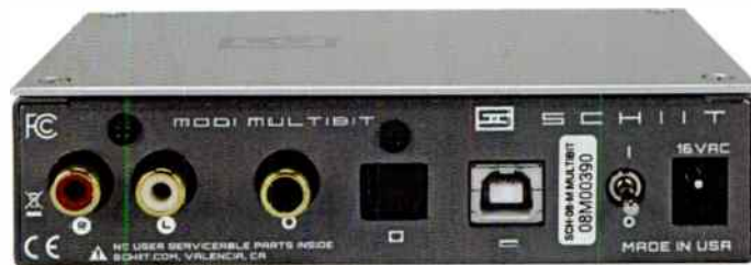
The rear of the Modi has digital co-axial, Toslink and USB-B inputs plus RCA analogue out sockets. A toggle switch turns the unit on and off.
