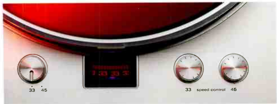
Two speeds, independent speed adjusters and stroboscope markings, visible through a small window. Speed is adjusted so the markings appear stationary.
