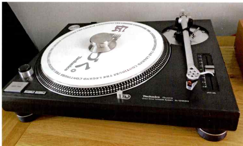
Technics SL-1210 Mk2 Direct Drive turntable fitted with Rega RB-310 arm, sitting on a Sound Supports arm plate – seen a rear right. "Nothing short of a revelation" says Ashley Garbett.
