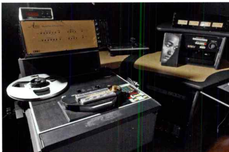
The Aria Class A electronics (created by the late Mike Sptiz) served as a necessary upgrade to the attached and refurbished Ampex tape recorder.
