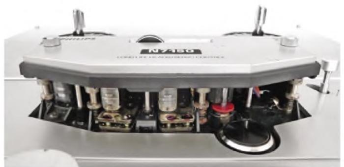
**The N7150 has a three-head configuration for the best performance and flexibility. To the right can be seen the pinch roller, which retracts when it's not required.**
