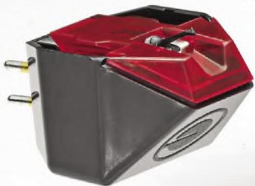
The E3 comes in at £99 and has the aluminium cantilever of the E2, but with an elliptical stylus to better retrieve high frequency information from the groove.
