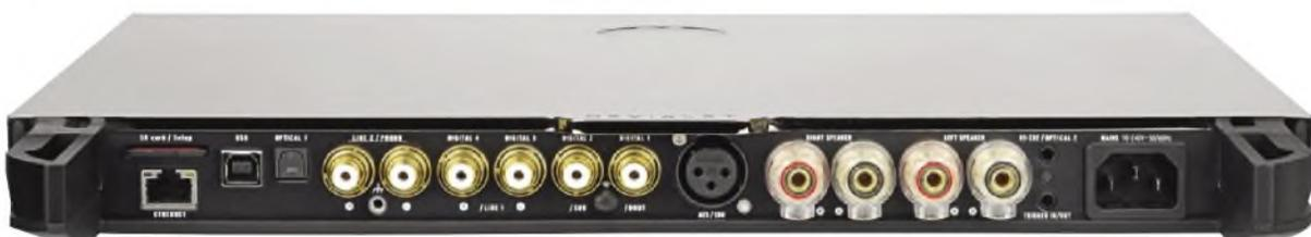
**Inputs on the back of the Devialet include analogue, digital Toslink and coaxial as well as AES/EBU. A USB connection also allows for file sizes up to 32bit/192kHz as well as DSD.**
