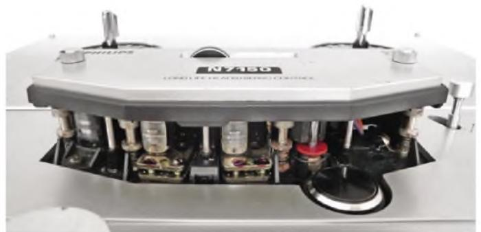
**The N7150 has a three-head configuration for the best performance and flexibility. To the right can be seen the pinch roller, which retracts when it's not required.**
