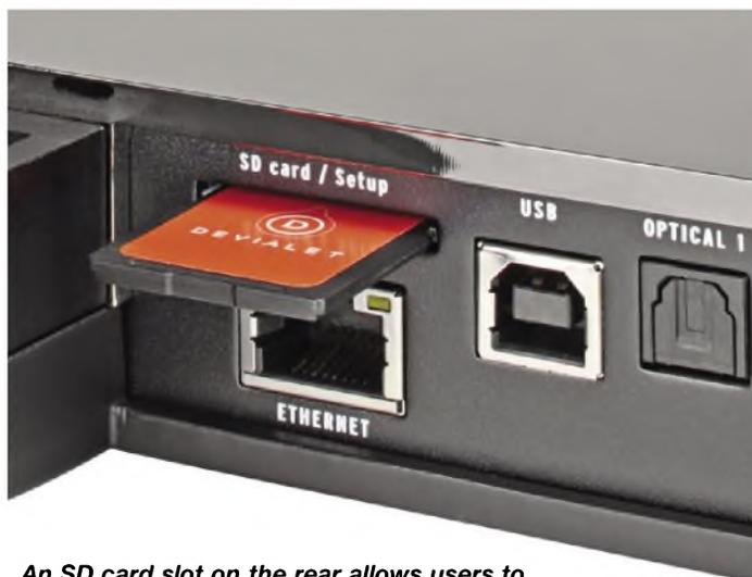
An SD card slot on the rear allows users to configure the amplifier to personal taste.
