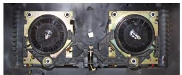
**The N7150's reels are driven by individual DC motors, which provide plenty of torque. This sort of arrangement, standard on more expensive machines, is rare on budget decks.**
