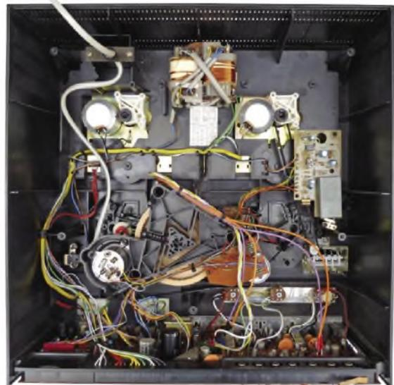
**Internally, the N7150 is more sophisticated than the Akai and Sony competition. There are two reel motors, a servo-controlled capstan motor and a fourth 'mode control' motor. The deck makes considerable use of fragile plastics to achieve low cost and light weight.**
