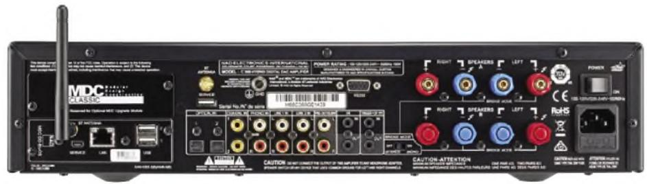
**The C368 is well-connected. There are four digital inputs, two analogue line inputs, a phono stage, provision for two sets of speakers and – for real power addicts – a bridging function.**
