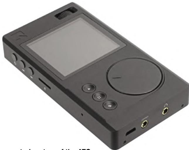
**The control system of the ATC features three buttons on the front with a scroll wheel while the volume control is at the top and fast forward/rewind and next track buttons are on the side. It's not the most elegant layout but works.**
