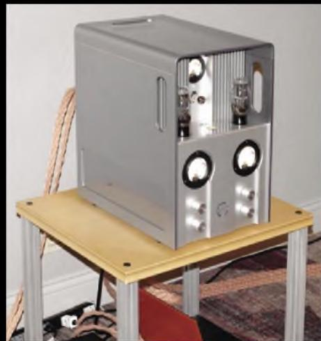
An industrial design idiom, with big open face meters, sturdy casework and exposed tubes (2A3 valves) made this Whammerdyne visually arresting. It uses direct coupled tubes and an output transformer to deliver 4 Watts, so sensitive 'speakers are needed.
