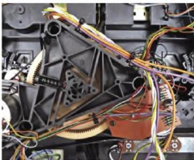
**This subchassis contains the flywheel, the central spindle of which surfaces as the capstan. It's belt-driven from a DC motor, which also contains the tachogenerator providing feedback to the speed-control servo system. Two of the three lugs that secure the subchassis to the body were found to be broken on my specimen!**
