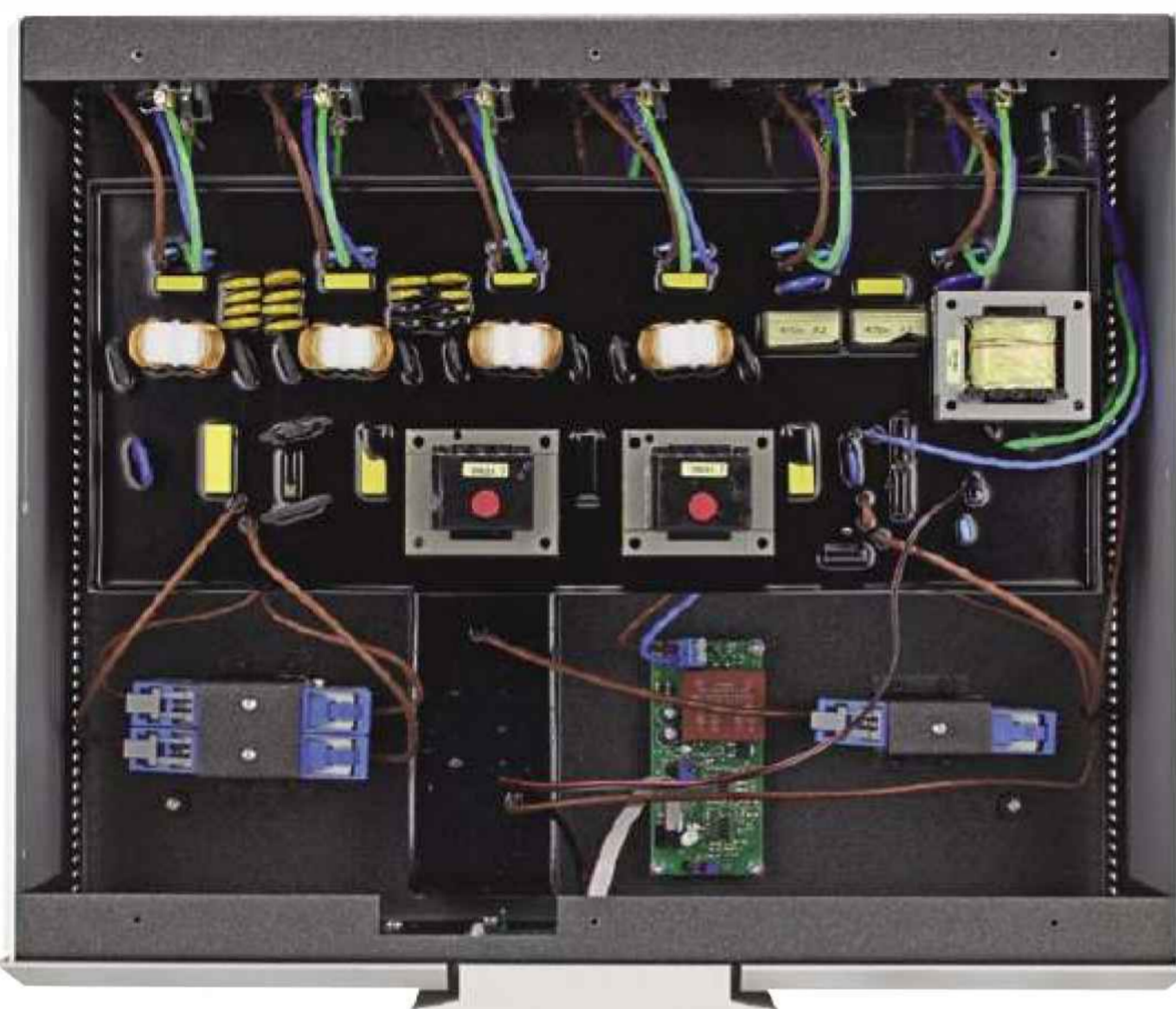
Each outlet has its own conditioner – there's an additional layer of filtering components not obvious in this photo. Note the use of pitch to damp vibrations.
