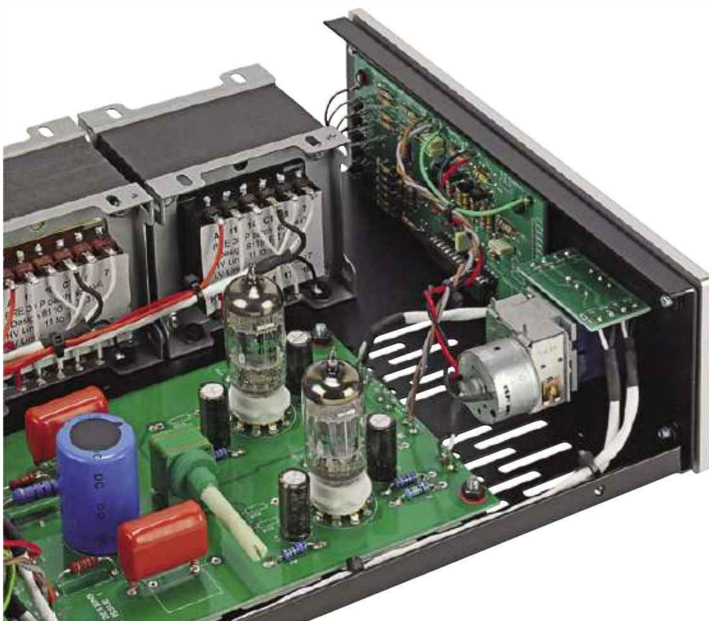
A clear view of the Alps motorised volume control (right), front indicator and input select board and massive line output transformers – expensive (so not used by anyone else).
