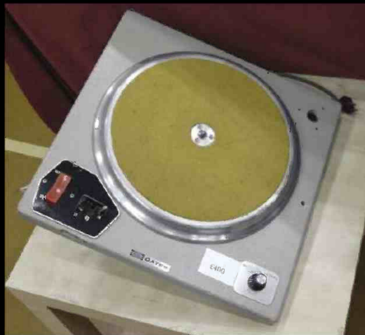
In the 1970s transcription turntables made by the U.S. Gates corporation were regular fixtures in broadcast studios around the world. This one is the CB77, which has a 12in. platter. The 'gearstick' speed change knob of this £400 specimen was removed to prevent it falling prey to the sticky-fingered.
