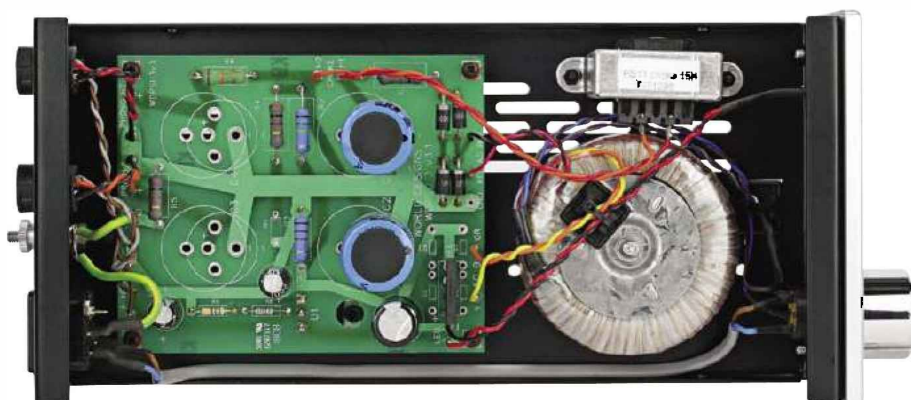
The power supply unit, PSU3, with toroidal mains transformer at right, frame choke (top), Schottky diode rectifier and smoothing capacitors.
