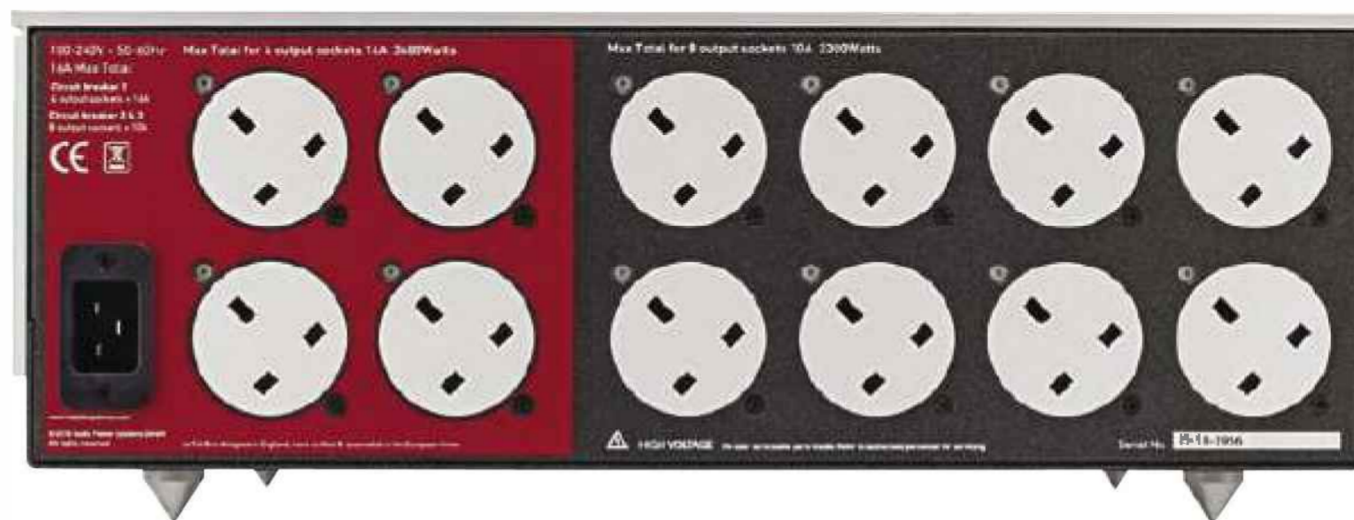
The outlets of the first B block of eight (black), rated at 10A, are intended for source equipment. Amplifiers and other hungry components plug into the A block (red), with four 16A sockets.
