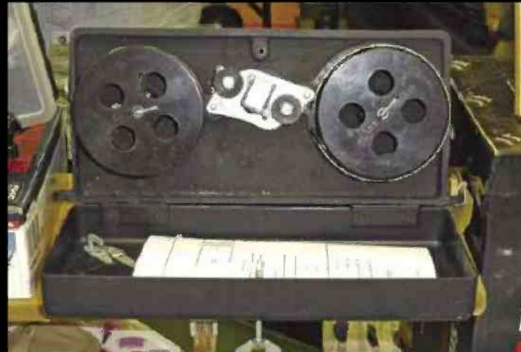
This well-preserved wire recorder, made by Boosey and Hawkes subsidiary Wirek, was claimed to have been stripped from a Lancaster bomber. Its electronics are built around a CV491 double-triode, one of the earliest B9A valves. A piece of history, for £80.
