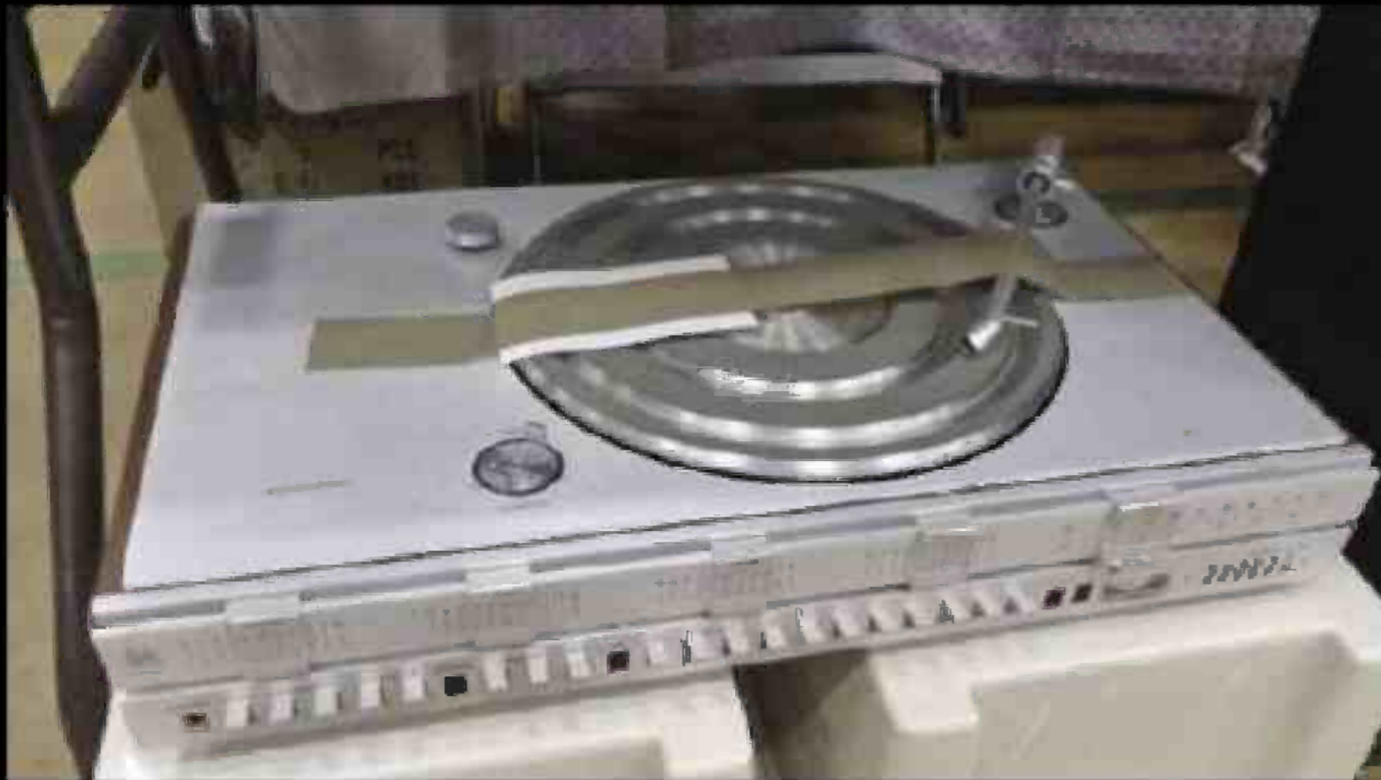
A Beocenter 3500, from Bang and Olufsen – a hybrid of the Beogram 3000 automatic turntable and 40 watts per channel Beomaster 3000 stereo receiver. This well-preserved example's tonearm is bereft of cartridge. B&O special cartridges are difficult (read: 'expensive') to obtain nowadays. Hence the modest £40 asking price...
