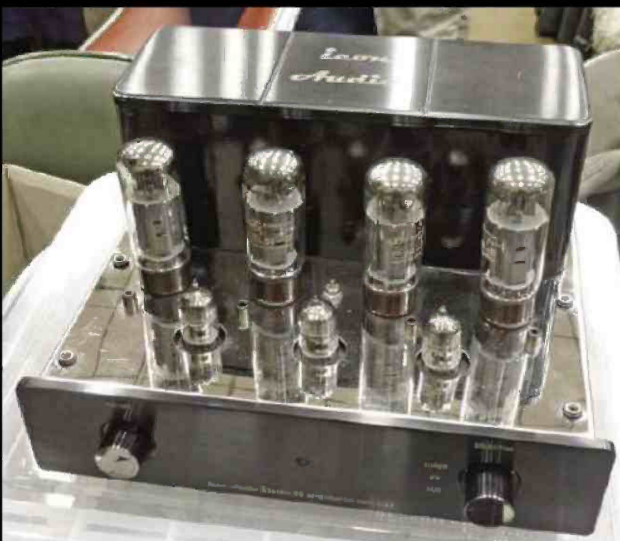
In the late noughties, Icon Audio brought out the Stereo 25. This is an affordable integrated amp based around EL34s working in push-pull. It holds its value too; this Icon 25, which originally sold for £500, was being offered here for £400.
