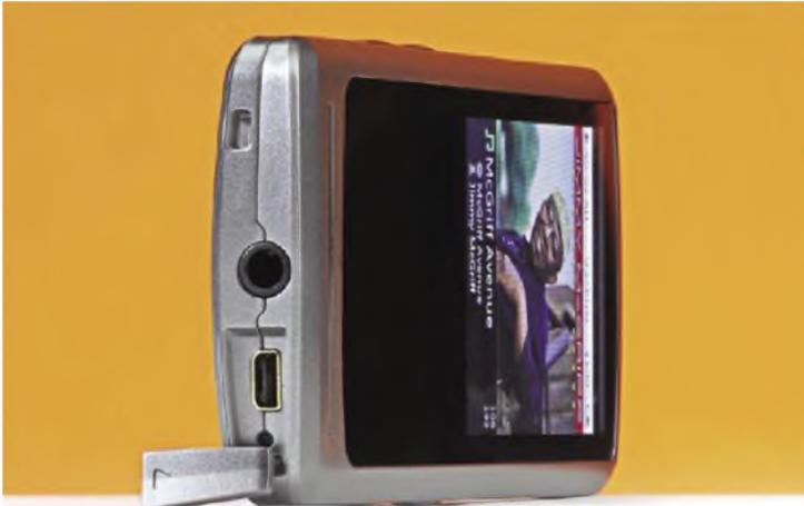
The underside of the Cowon has a 3.5mm headphone socket, plus a USB socket for importing tracks and charging.
