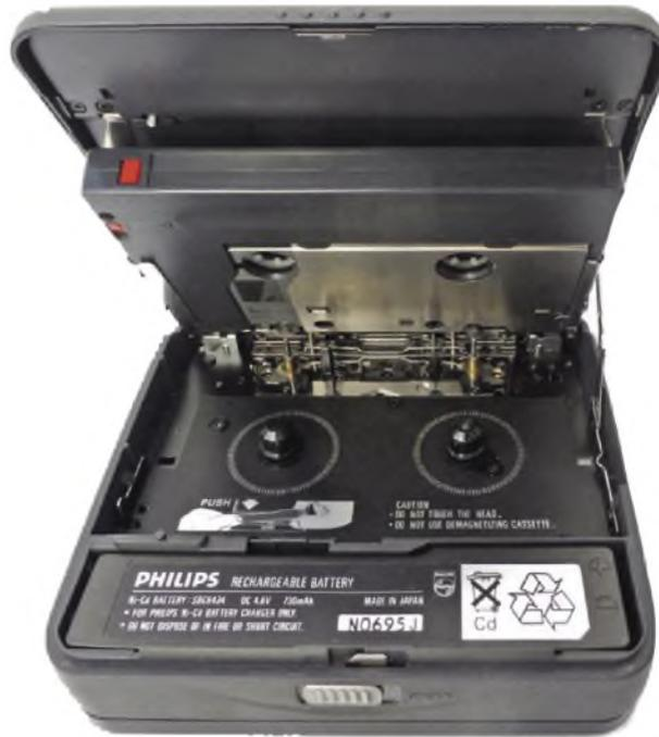
**Looking into the jaws of the DCC170 mechanism, showing how a DCC cassette is loaded. Obscured are the magnetoresistive head assembly and pinch-rollers, although the capstan drive shafts can be seen. In front, the battery compartment; the DCC170 runs for up to three hours from a 720mAh rechargeable NiCd battery – visible. The 4.8 Volt battery can be removed and replaced if necessary.**
