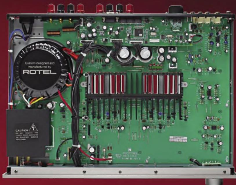
*Under the toroidal mains transformer (top left) is a small standby one. A daughter board contains the remote-control circuitry, Bluetooth DAC and control microprocessor chip. A front-panel rotary encoder controls volume.*
