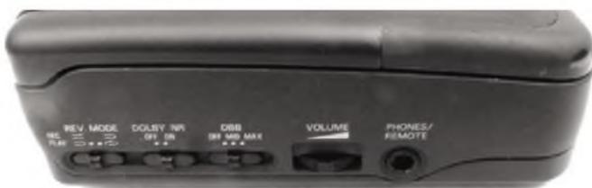
***Philips has managed to cram connectors and switches onto just about every surface! The left side has controls for auto-reverse mode, Dolby B for analogue cassettes and the bass-boost function that was at the time apparently obligatory on all Walkman-type devices. Here too is the volume thumbwheel, and a headphone socket that also accepts an inline remote ‘dongle’ (an essential accessory for bootleggers!).***
