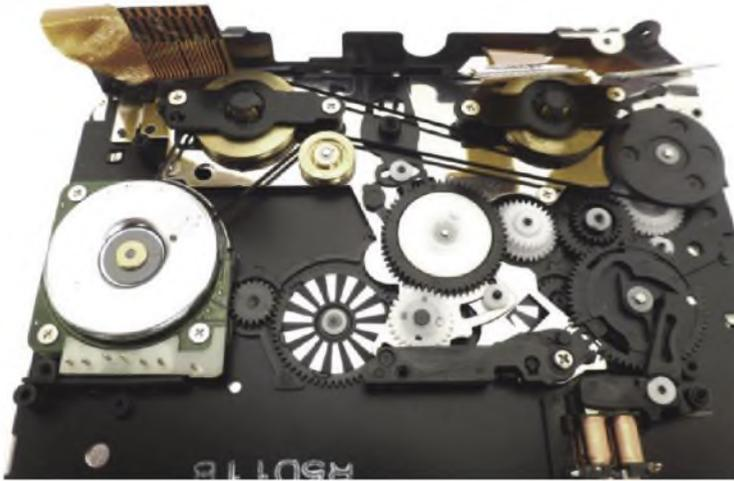
*If you take apart a DCC170 in order to replace its drive belt – an involved task that should be avoided by the faint-hearted, not least because a soldering iron is involved! – this is what you’ll see. The whole shooting-match is controlled by the motor and solenoids, all of which are under the control of the DCC170’s microprocessor. The ribbon cables go to the head assembly.*
