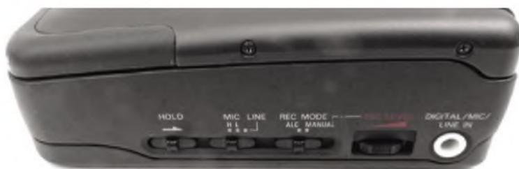
**On the other side is a switch that switches the analogue input – the 3.5mm connector also accepts optical digital audio from a CD transport or similar unit – between microphone and line sensitivity.**
