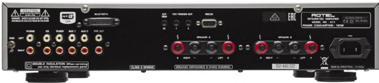
Four line-level inputs, plus an input for MM cartridges, complete with earthing post, and a pre-amp output. The latter, which are affected by volume/balance and tone controls, are for bi-amping or active speakers. You can also see here the remote connections, Bluetooth aerial and the two sets of independently switchable speaker outputs.
