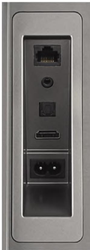
**Underneath lies the power input, wired internet connection, analogue input via 3.5mm stereo jack and optical S/PDIF digital input.**
