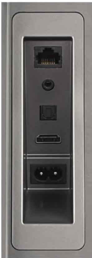
**Underneath lies the power input, wired internet connection, analogue input via 3.5mm stereo jack and optical S/PDIF digital input.**
