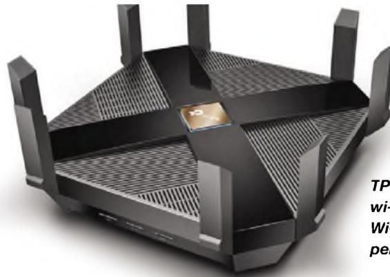
**TP-Link Archer AX6000 wi-fi router capable of Wi-Fi 6 (802.11ax) performance.**
