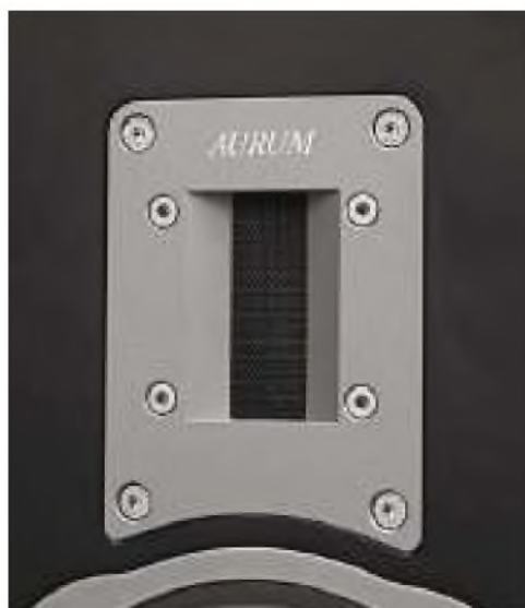
Quadral's ribbon tweeter sits close to the midrange unit for good phase matching, to give a consistent sound at different listening (ear) heights.
