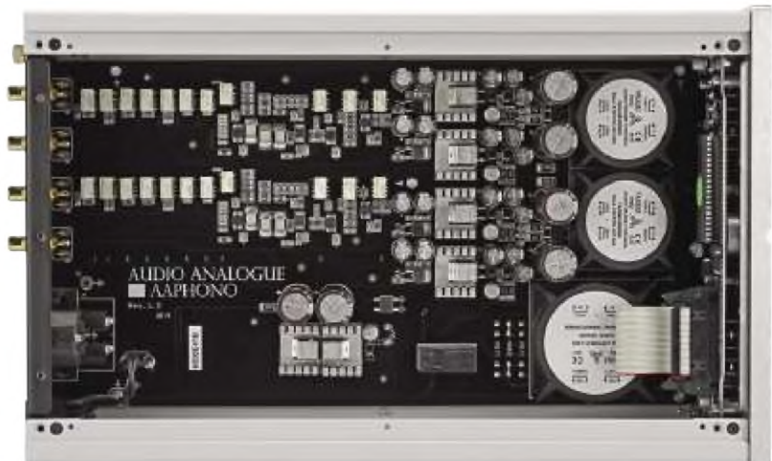
The AAPHono majors on linear power supplies, having no fewer than three mains transformers, seen at right. Two supply power to each channel, the third power to the switching circuits and ancillaries.
