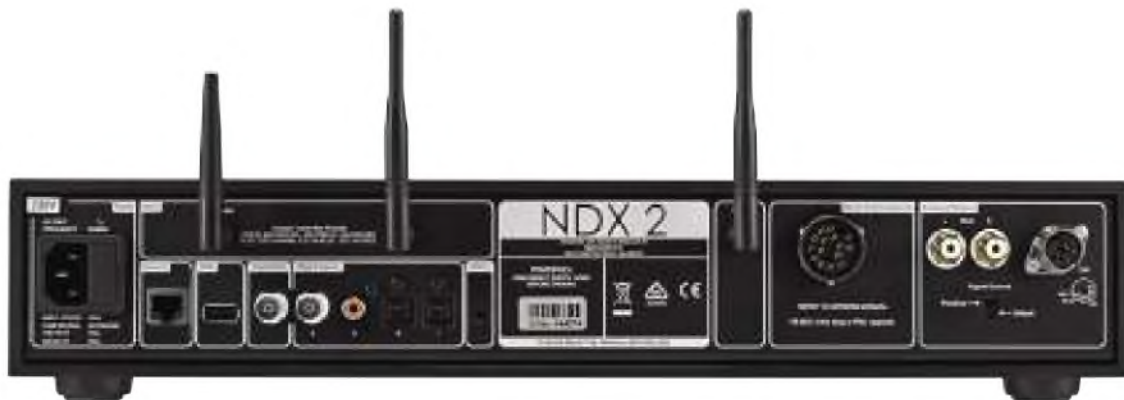
Two external wi-fi aerials and one Bluetooth aerial help make the NDX 2 sensitive to household router and phone signals, aiding data speeds and reception stability. There is an array of digital inputs and Naim's DIN socket output at right, but no XLR balanced outputs from the DAC.
