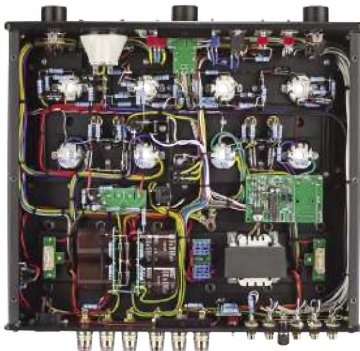
A hard-wired internal assembly, with neat wiring looms. There are also printed circuit boards for remote control etc, two fuses (bottom left and right), plus a big choke (bottom right) to clean the power rail. It is a specialised and expensive component.
