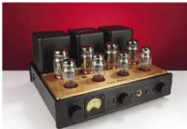
Icon Audio Stereo 40 MkIV valve amplifier. "Design the audio circuitry with a carefully calculated rising output as the frequency rises" to fix its warm, no-feedback sound, suggests John Malcolm.
