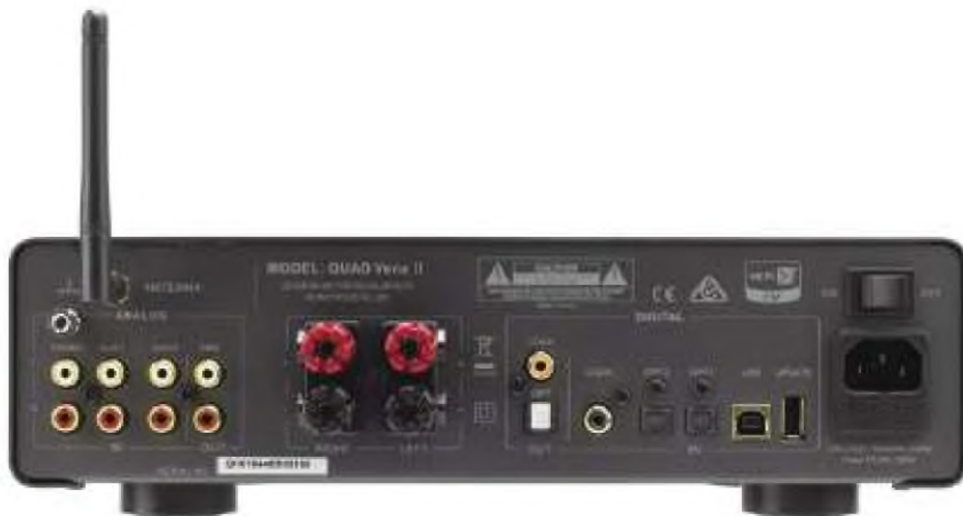
It may look bare and the 'speaker terminals basic, but there are a lot of inputs on the rear panel, from analogue turntable (MM) at left through to digital USB at right, plus an aerial for Bluetooth.
