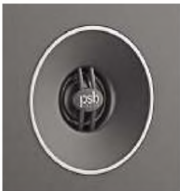
The proprietary 0.75" (19mm) black anodized aluminium dome tweeter sits in a shallow wave guide and has a phase plate in front to smooth response.
