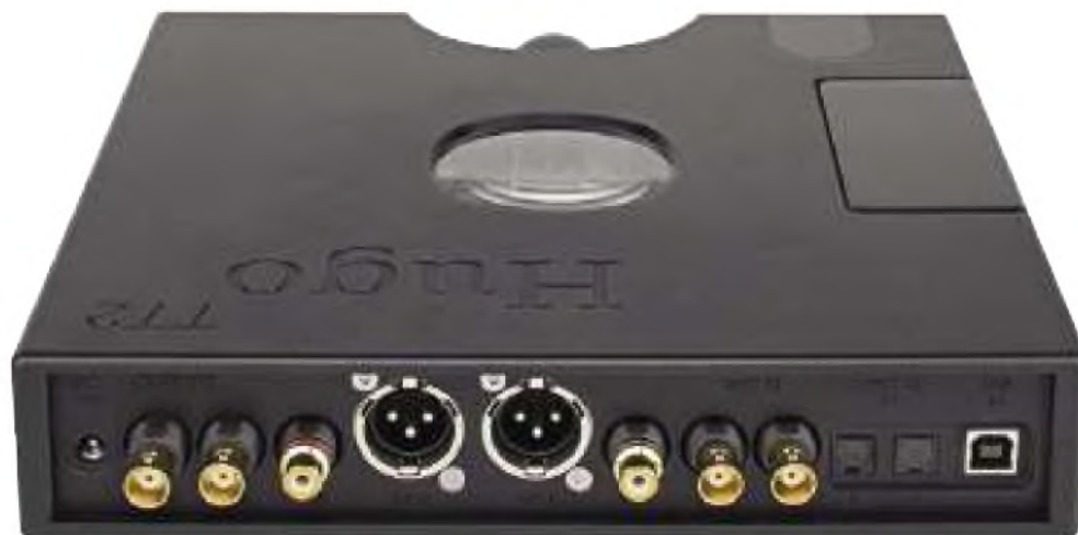
At left, twin BNC output sockets (for future products). Next along, two large XLR socket outputs flanked by phono-socket outputs. Then come twin BNC digital inputs that together form a DBNC input. At right are TOSLINK optical inputs and a USB B computer connection.
