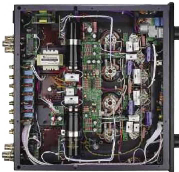
A complex internal layout with hard wired white ceramic valve bases, a central green circuit board and – at left – gold plated input sockets switched by relays. At top right is the Alps volume control, motorised for remote control operation.
