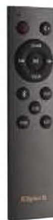
The remote selects sources, changes volume, mutes the sound and selects standby. It is a bit of an ugly duckling compared to the Three II.
