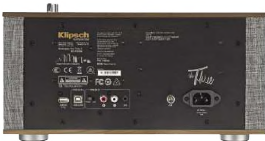
The Klipsch Three II rear panel carries a USB socket for computer audio (up to 192kHz/24-bit) but conventional digital sources aren't catered for. A slide switch converts the phono-socketed line input into a Phono input for a turntable.
