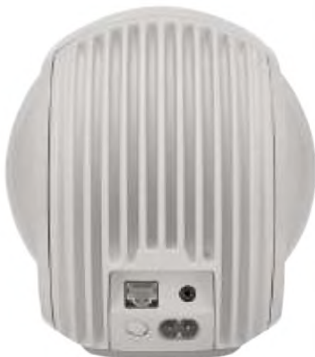
At rear is the wired ethernet connection, power supply socket and a 3.5mm analogue/digital (optical) input jack.
