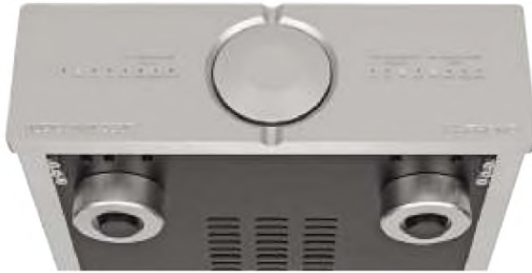
Just beneath and behind the front fascia plate lie small black push buttons, at left and right. They select MM or MC gain, plus loading values for MM and MC cartridges.
