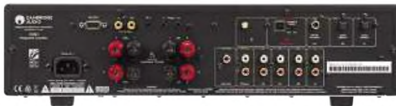
The rear panel includes RCA phono socket analogue inputs as well as co-axial and optical digital sockets, but no balanced XLRs.
