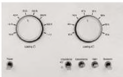
Top panel controls. At left is a rotary MC ( \Omega ) load switch and at right an MM ( k\Omega ) load switch. Lever switches below select MM capacitance, gain and Subsonic filter.
