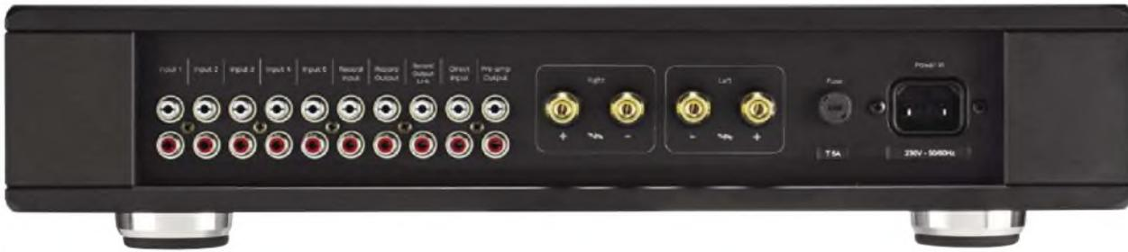
The rear panel offers five line level inputs, plus tape in and out and a preamp output, all through RCA phono sockets. One set of loudspeakers only, so no loudspeaker switching. No balanced inputs either.
