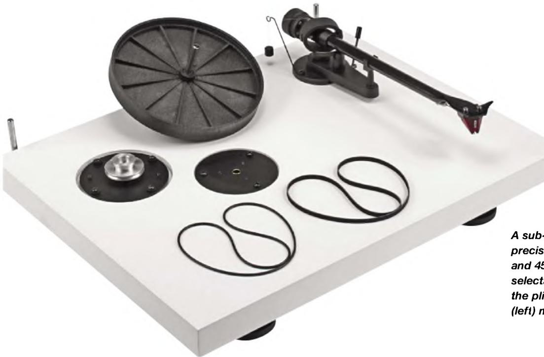
*A sub-platter is driven by a precision flat belt for 33rpm and 45rpm speeds, switch selectable at front – beneath the plinth. A simpler O ring belt (left) must be fitted to spin 78s.*
