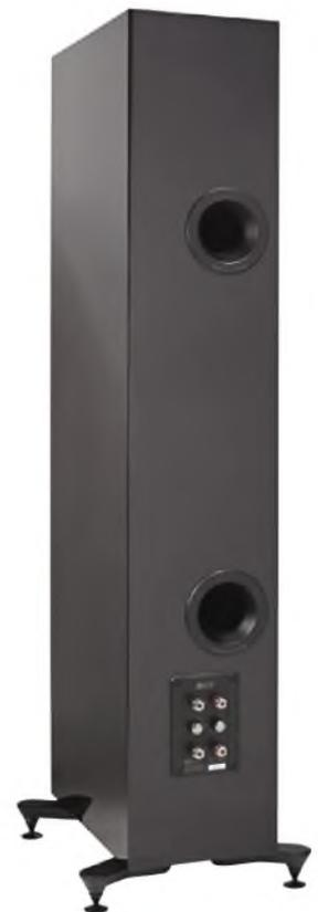
**Upper and lower reflex ports tune the internal bass chambers slightly differently, to smooth low bass and give an even amplifier load.**
