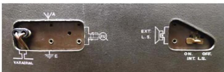
**Separate aerial inputs are provided for AM (medium/long-wave) and VHF. A matching transformer, known as a 'balun', is necessary for an external rooftop VHF/FM aerial.**
