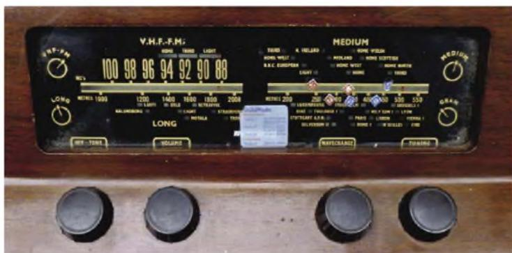
**Four knobs cover tone/power off, volume, wavechange/gram selection and tuning. The backlit side-by-side tuning scales are marked with stations. Right covers medium-wave, left covers VHF-FM and long-wave.**
