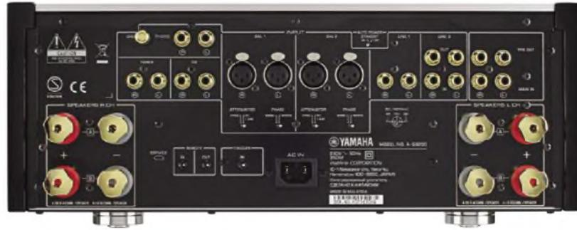
**The rear carries two sets of balanced Line inputs via XLR sockets (top centre) with attenuator and phase selector switches. Two sets of loudspeakers can be used, or both turned off for headphone listening, or both turned on for bi-wiring.**
