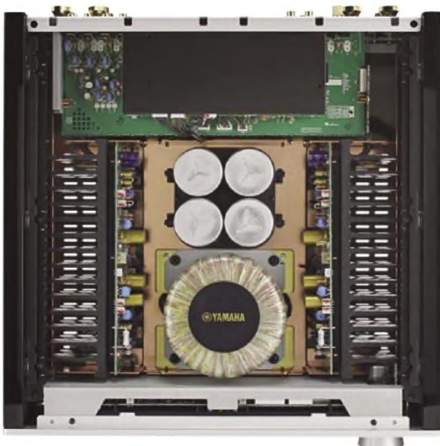
**A massive toroidal mains transformer with smoothing/reservoir capacitors dominates the top view. The power boards sit next to the heat sinks at left and right, in classic arrangement.**
