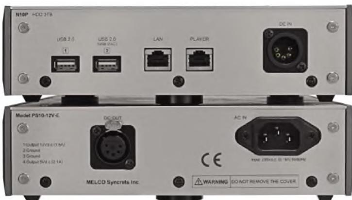
**At bottom the linear power supply with its multi-pin Neutrik power output socket. At top the N10 'head unit' with USB sockets for mass storage and USB DAC connection. There's an ethernet link to router and one direct to Player.**
