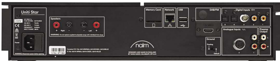
The rear has 4mm loudspeaker sockets for banana plugs only; Naim supply custom plugs to fit. At centre RJ45 ethernet and USB mass storage sockets. Digital and analogue inputs at right, including a DIN input and a Phono input for a turntable. All analogue is converted to digital.
