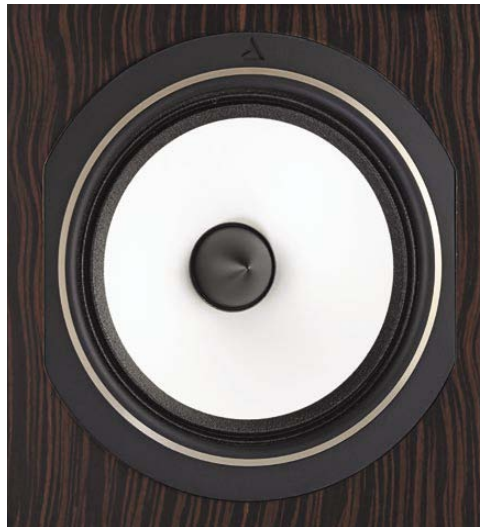
Triangle's large, white midrange unit, made of uncoated cellulose paper, covers much of the audio band. At centre lies a stationary phase plug to prevent interference at the cone base.
