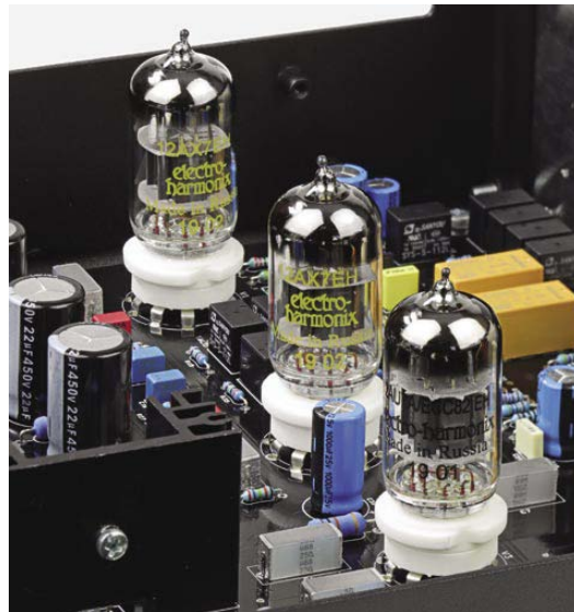
Two Electro Harmonix 12AX7 (ECC83) double-triode preamp tubes and one ECC82 (12AU7) cathode follower output tube provide amplification for MM cartridges. JFET transistors provide further amplification for MC cartridges.
