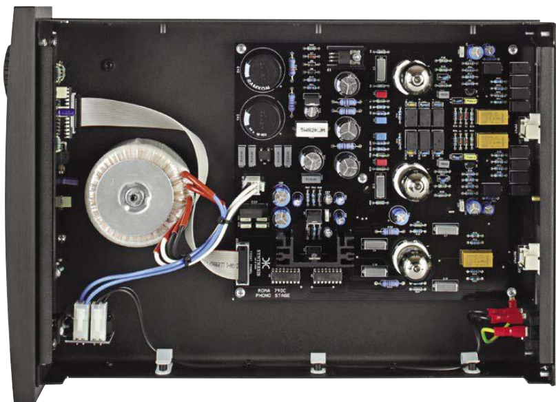
From above the Roma 79DC looks dense and complex. At left its toroidal mains transformer is able to deliver high voltage to the valves, through on-board power supply circuitry. Discrete components and small-signal relays are used for best sound.
