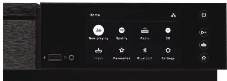
The front panel screen carries a comprehensive display of inputs, sources and settings. There's a USB mass storage socket and 3.5mm stereo headphone jack too.
