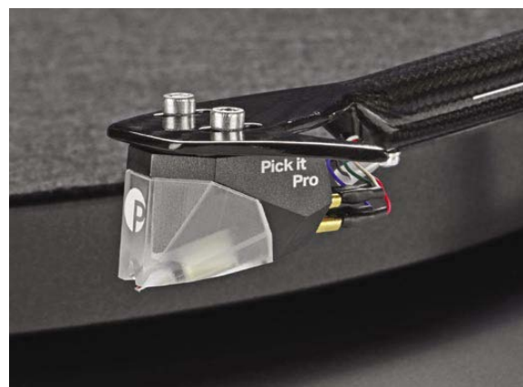
A flat finger lift makes hand-cueing difficult. Too close to the LP for a finger – and too slippery too!
