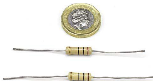
Two 1W carbon film resistors, ideal for attenuating the treble of a bi-wire loudspeaker. Use 1Ω or 2Ω total (not 10Ω shown here).
