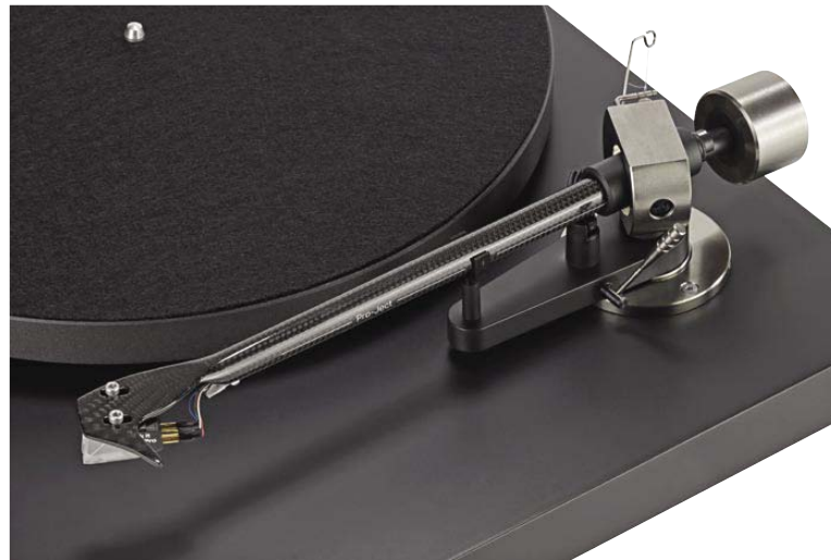
The one-piece wrapped carbon fibre arm is light and its tube rigid, but undamped and resonant. The rear counterweight is uncalibrated so a stylus force gauge is essential.
