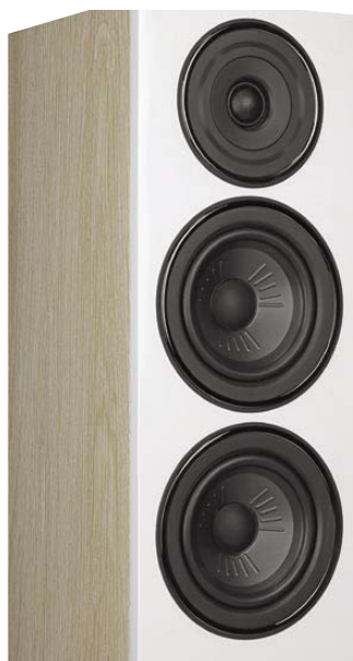
The two bass/midrange drive units have ribs to add stiffness and break up waves. The black cone material is a polypropylene/mica composite.
