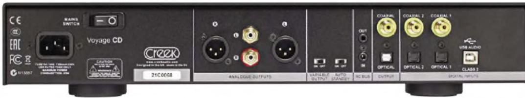
At centre the analogue signal outputs, and at far right the digital inputs, including USB. There are also optical and electrical digital outputs from the transport.
