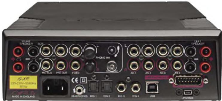
**i9-XR offers analogue inputs, an MM phono input, a USB input and four digital inputs (2 x SPDIF, 2 x optical). It also provides a headphone output and a multi-pin for the separate PSU-XR power supply upgrade.**
