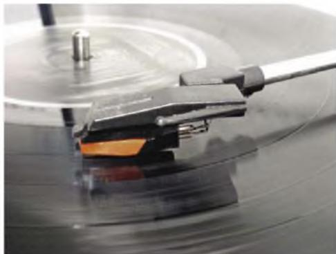
**The Cruiser's stereo ceramic cartridge is hardly in the same league as, say, the Decca Deram. Some claim it tracks at weights as high as 10 grams!**
