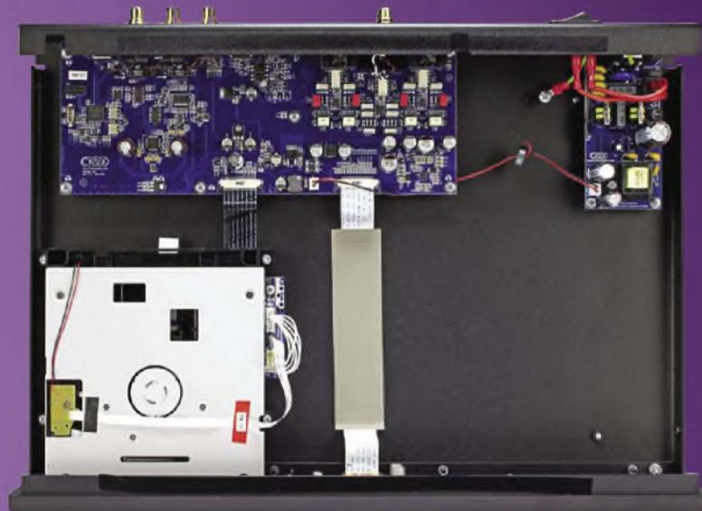
*At bottom left the Stream Unlimited slot loading mechanism that connects via ribbon cable to the main board housing an AKM DAC. At top right a small switch-mode power supply board.*
