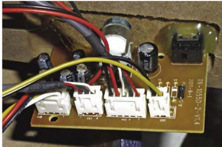
**The Cruiser's front-mounted speakers are powered by a TDA2822 stereo amplifier chip, which lives on this small circuit board. An 8-pin chip, it can be driven directly from the cartridge with no need for the additional gain of a preamplifier stage.**
