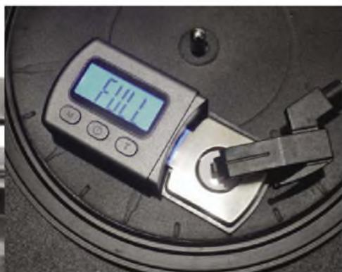
**The tracking force of the Cruiser's cartridge evidently exceeds the 5 grams limit of this stylus pressure gauge! Not good for record life.**
