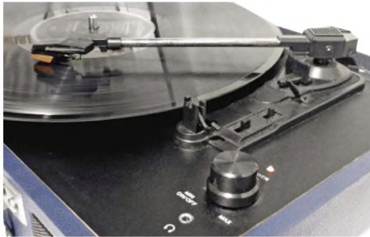
**The Cruiser, let loose on a copy of David Bowie's Scary Monsters LP. The tonearm, as we can see, is tubular and straight - not so obvious from this photo is the significant amount of 'play' in the pivot bearings.**
