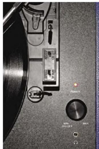
**A vertical slide-switch to the right of the tonearm changes the platter speed between 33, 45 and 78rpm; beneath it is another slide switch that removes power from the motor whenever the tonearm isn't positioned over the record's playing area.**
