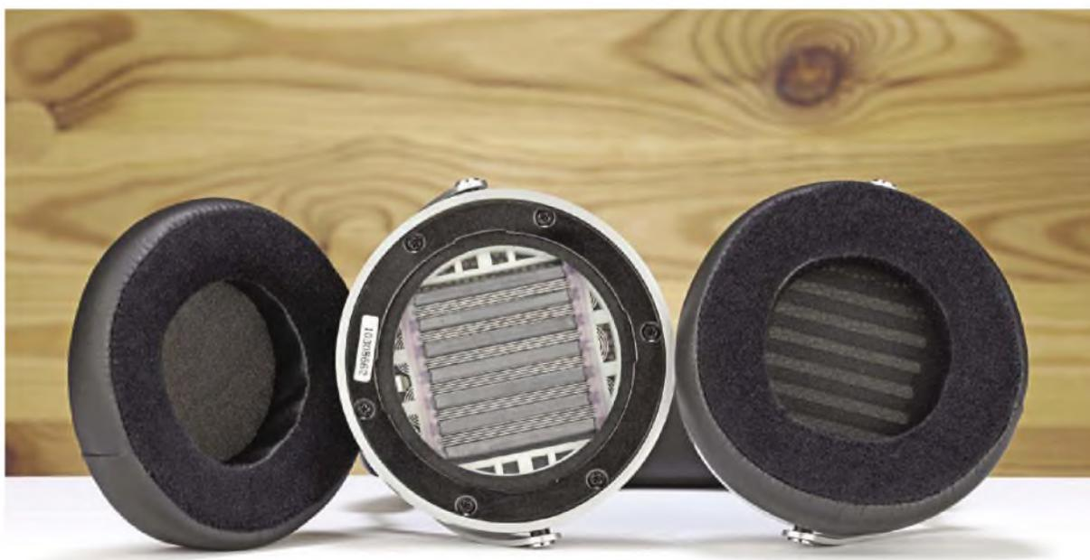
*At centre, the planar drive unit with its bar magnets in front of a mylar film embossed with current carrying tracks, to produce sound from a signal. The earpiece at left simply twists on to give the complete assembly seen at right.*
