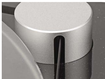
Teac supply a neat cover for the motor pulley. It must be aligned to avoid the belt.
