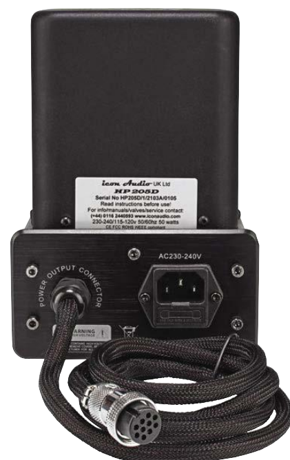
A conventional IEC mains input socket, plus sturdy output cable with 10-way socket.
