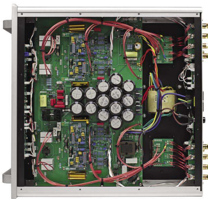
From below the Reference 80S power amplifier board is packed with smoothing capacitors (centre), safety fuses and special parts. At right is the mains transformer (yellow) and – above and below – output transformers with connection boards.
