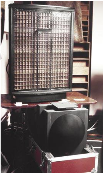
Polygram Records used stripped down Quad ESL-63s and Celestion SL-6000s driven by Celestion's equaliser.
