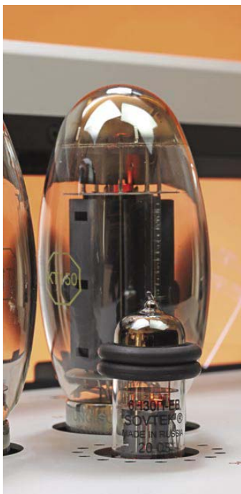
Behind, a KT150 power output valve. In front a 6H30 double-triode with damping rings.
