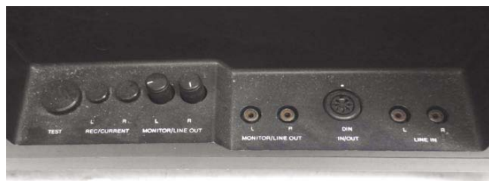
A legacy DIN connector was fitted, plus recording calibration and output level controls. Mechanical pushbuttons meant that remote control was not possible.
