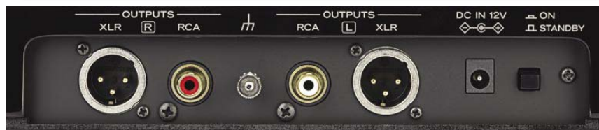
At rear are balanced XLR outputs and isolated (balanced) phono socket outputs. The earth terminal grounds the arm, as do the XLRs via Pin 1.
