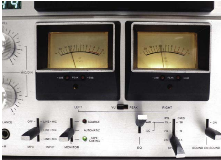
The large, wide-range meters are switchable between VU and peak characteristics. LEDs indicate peaks of +3dB and +6dB.
