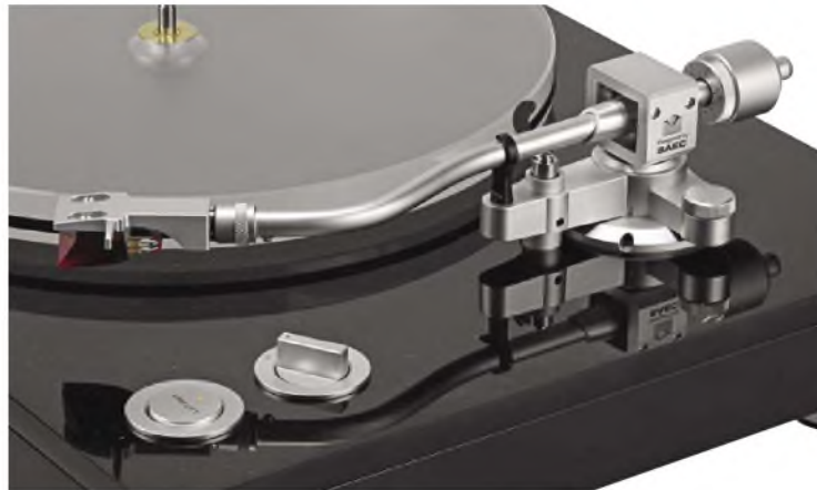
At front sits a circular lift/lower button with light touch action and small red LED to signal Up. Behind it lies a rotary speed selector.
