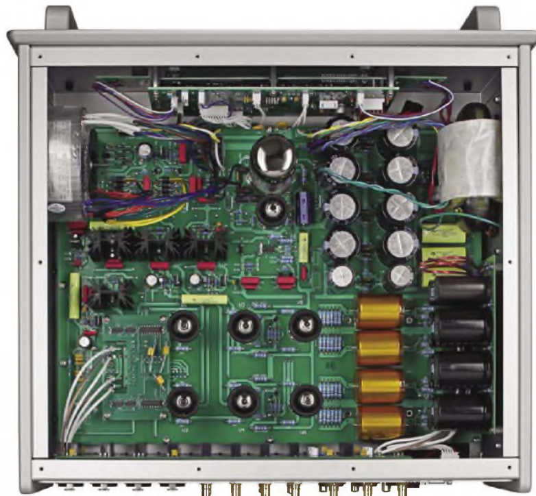
A top view of the 6SE preamplifier with clear acrylic cover removed. At right a C-core mains transformer, and at top centre 6550 and 6H30 valves to provide power regulation. Six 6H30s provide balanced amplification.
