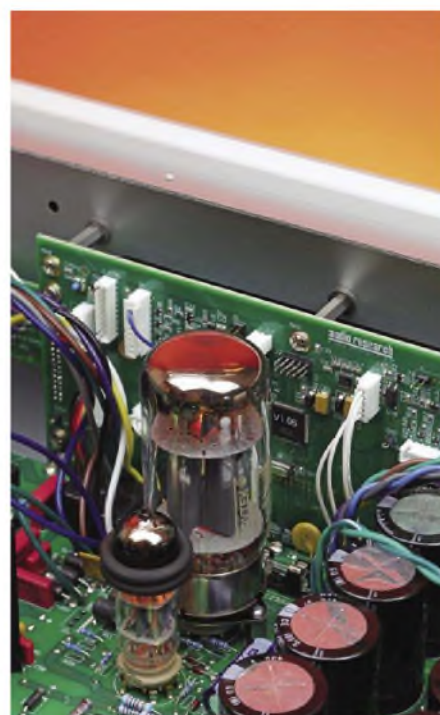
The 6SE has a valve regulated power supply for better sound quality. It comprises a 6550 power valve (rear) and smaller 6H30 double triode.
