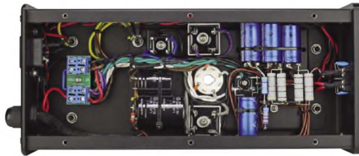
The power supply carries heater rectifiers (centre), a valve HT rectifier, and a supply for Bluetooth and DAC boards.
