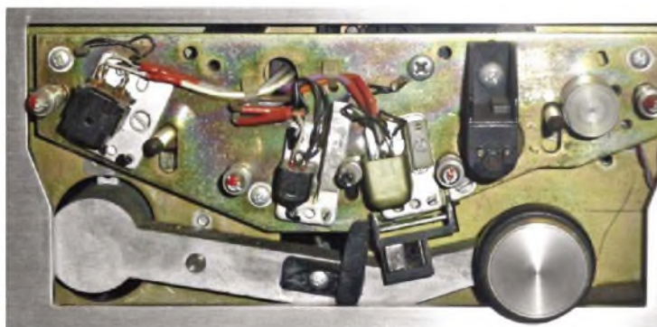
The record and playback heads are of parabolic profile for improved performance. Philips specified its own FSX material for the tape contact surface but it was not as robust as Japanese alternatives.
