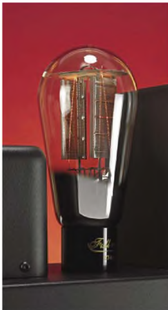
The 274B rectifier stands high and glows brightly. This is an optional extra.
