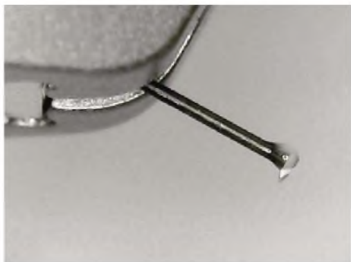
The diamond cantilever with diamond stylus bonded direct at 90 degrees.
