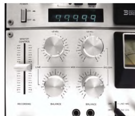
The stereo balance and levels of the line and mike inputs are independently-adjustable, allowing mixing and panning. A master slider allows the resulting combination of signals to be faded.
