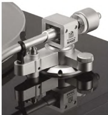
Height adjustable arm and lift platform; keys are supplied. Bias is set by a small rotary dial.
