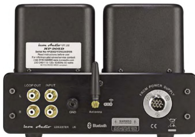
At rear, analogue input and loop-through output. An earth terminal and stubby Bluetooth aerial. At right a 10-pin input socket for power.
