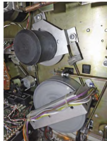
The N4520's hefty flywheel – coupled to the capstan that moves the tape – is belt-driven by a quartz-referenced motor. There are 9.5, 19 and 39cm/s speeds.
