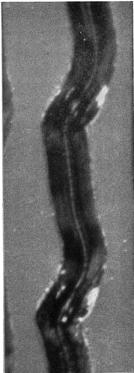
Fig. 4 —Another copy of LK4170 from the same master, showing the same (approximate) 1,000 c.p.s. piano note. This time the disc has been played 20 times with another pickup with a downward stylus pressure of 7 grams. The alteration of the groove can be seen quite clearly.
