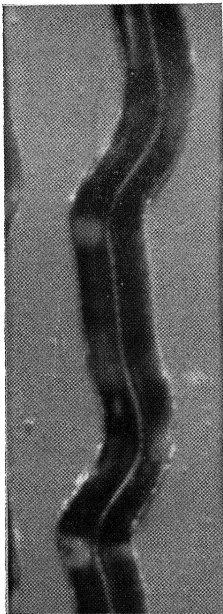
Fig. 3 —Here we see the same groove approximately (1,000 c.p.s. fundamental) of the same piano note, but the details of the scenery have changed quite considerably. The disc which was fresh from the press in Fig. 2 has now been played 20 times by a pickup with a downward pressure of 3 grams.
