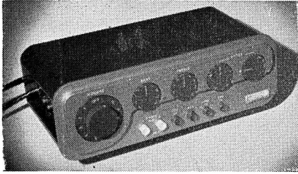
Quad II control unit
