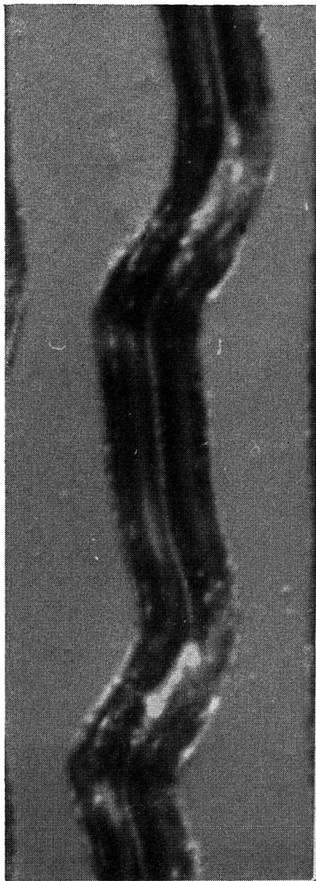
Fig. 5 —This disc (another copy from the same master), has been played 20 times by a 4-gram type pickup which required a downward pressure of 10 grams before it would track the groove correctly. Readers who are now horrified by the chaos may console themselves by the fact that this scenery is magnified \times 300 !
