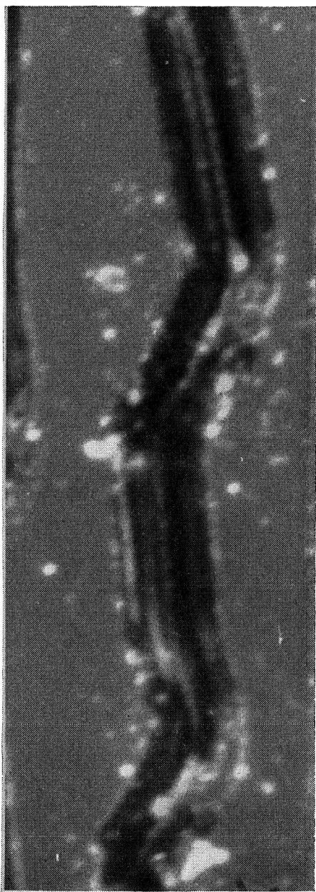
Fig. 6 —More chaos here! This picture was taken before cleaning the disc for photography. It is, in fact, Fig. 5. The "snow" is ploughed-out disc material. The moral is clearly emphasised—keep them clean; for whatever is in the groove is bound to colour the sound that emerges from the speaker.
